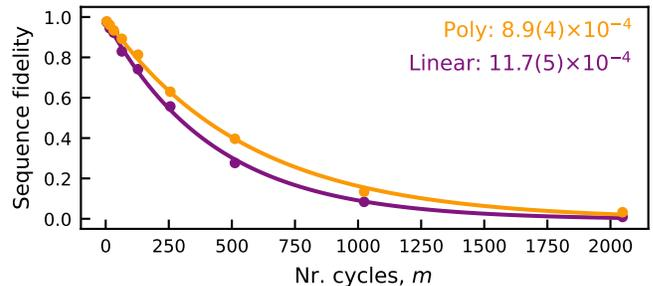
FIG. 4. Cross-entropy benchmarking (XEB) of random-angle single-qubit  $X$  rotations. The data points show the sequence fidelity, and the line is an exponential fit to the data. The legend indicates the total gate error obtained when using linear (purple) and polynomial (orange) scaling for calculating the amplitudes of the  $X$  pulses.
