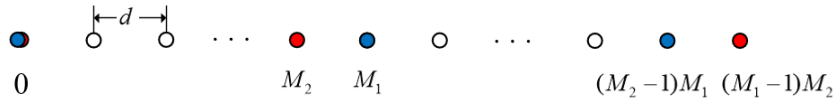
FIGURE 2 Schematic diagram of coprime array. ●: array element of subarray 1 ●: array element of subarray 2 ○: vacant array element
