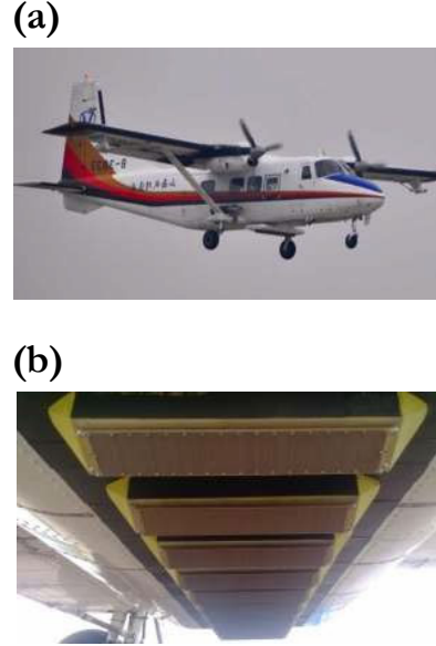
FIGURE 10 Array InSAR flight platform and antenna. (a) Array InSAR flight platform. (b) Array antenna.
