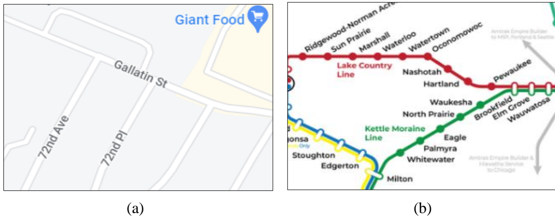
Figure 2. Representation of road networks labeling: (a) shows the labels within roads; (b) shows a railway network with labels around the line features.
