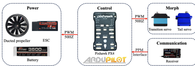
Fig. 3. Robot electrical schematic diagram and its wiring overview.
