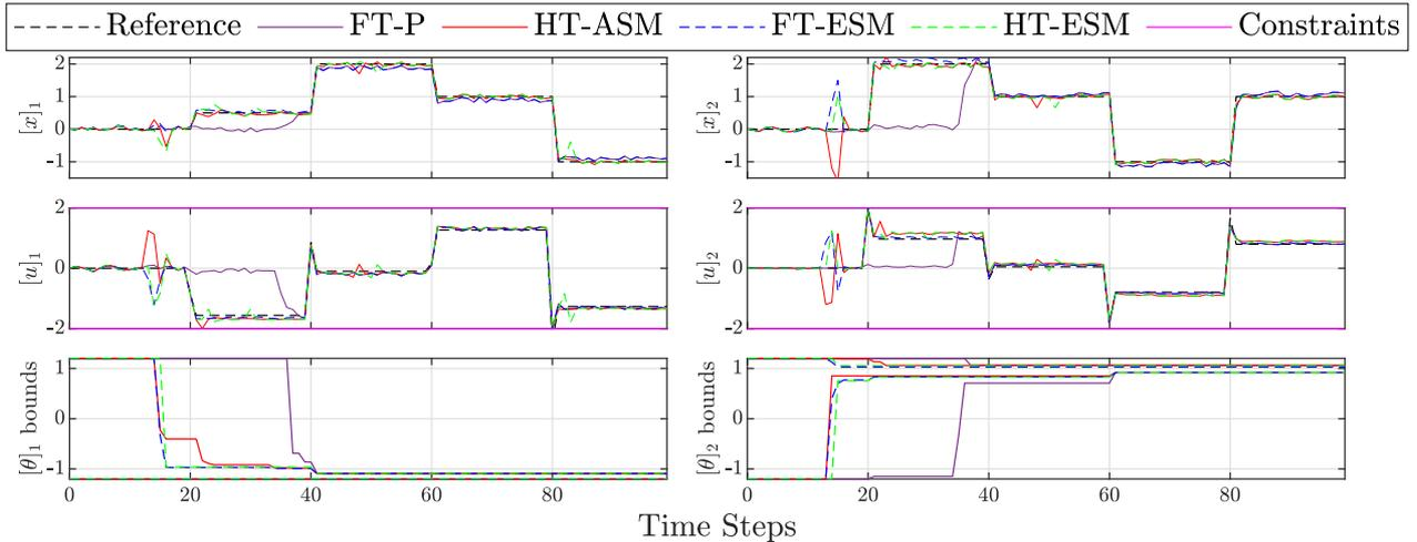
Fig. 2. State and input trajectories of the system under four different controllers, along with upper and lower bounds on parameters. The true parameter is  $\theta^* = [-1.16, 0.96]$ .
