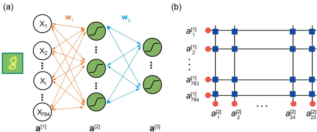
**Figure 6.** (a) Structure of a three-layer neural network. (b) Illustration of the crossbar resistive array between the input layer and the hidden layer, where the resistance of blue squares represents the weights and the red circles denote the neurons.
