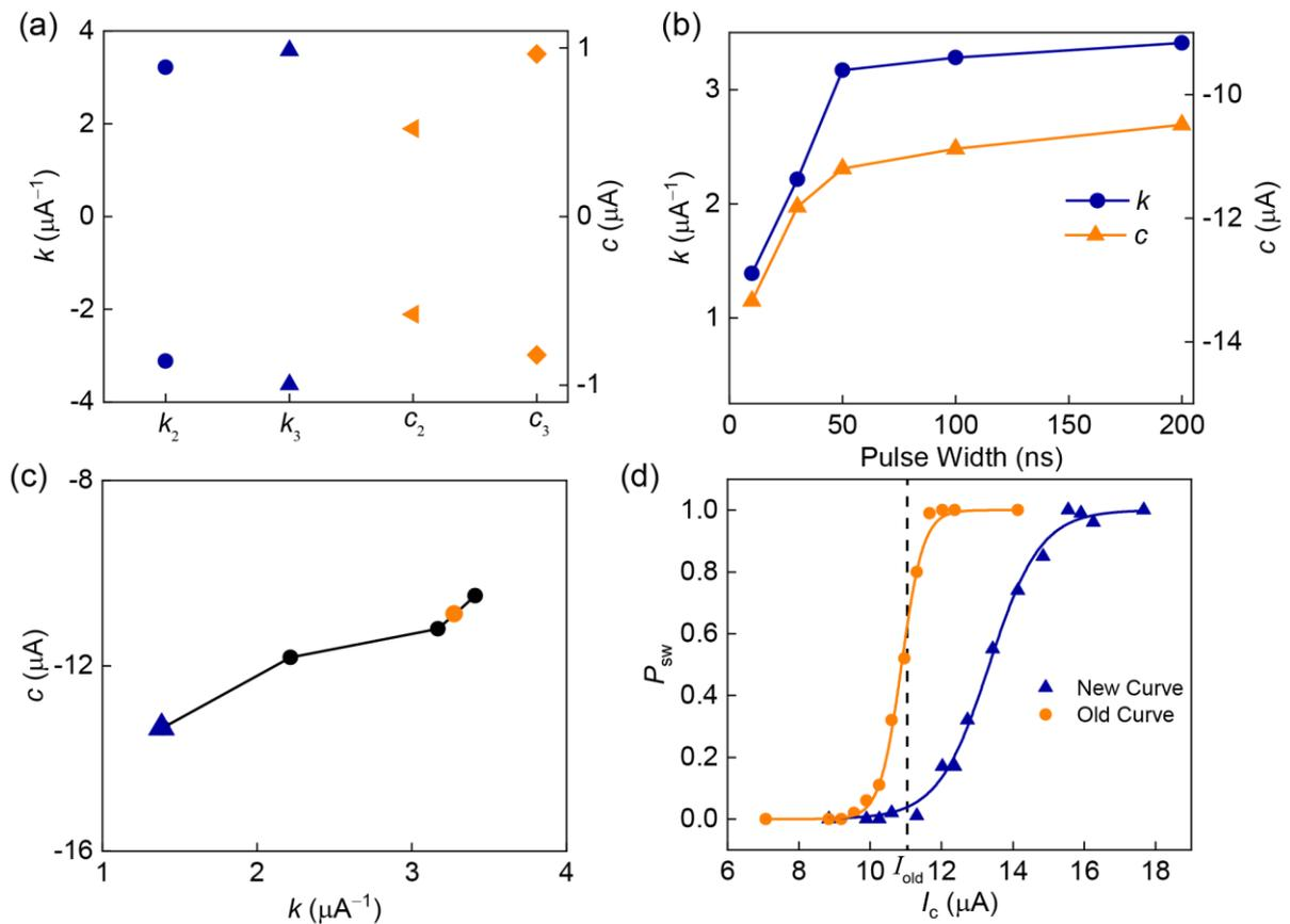
**Figure 2.** (a) Maximum ranges of  $k_2$ ,  $k_3$ ,  $c_2$  and  $c_3$  extracted from the software training. (b) Physically allowed  $k$  and  $c$  under different pulse widths. The values are extracted from Fig.
