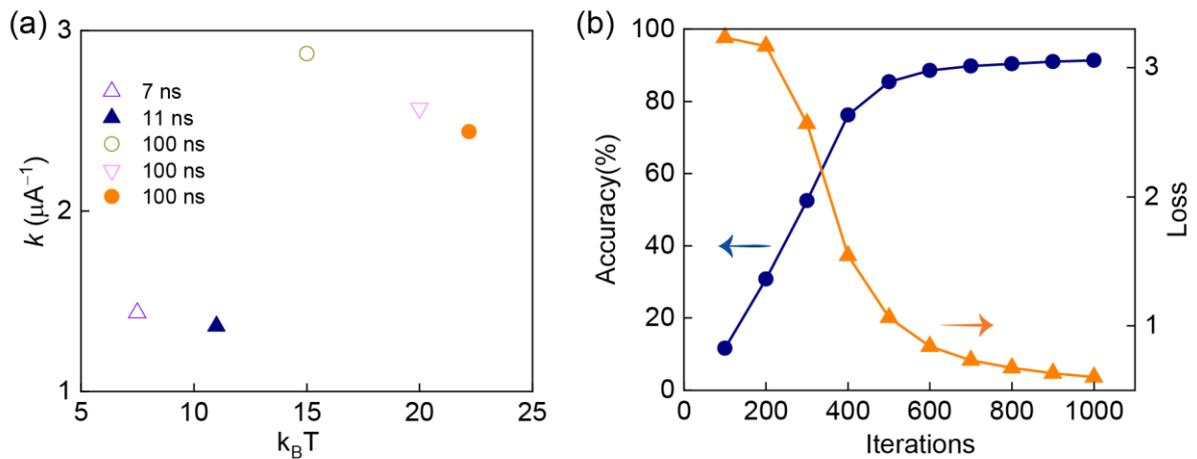
**Figure 4.** (a)  $k$  under different combination of  $E_B$  and pulse widths. (b) The evolution of loss
