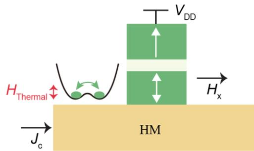
**Figure 8.** Illustration of the three terminal device combining SOT and VCMA.
