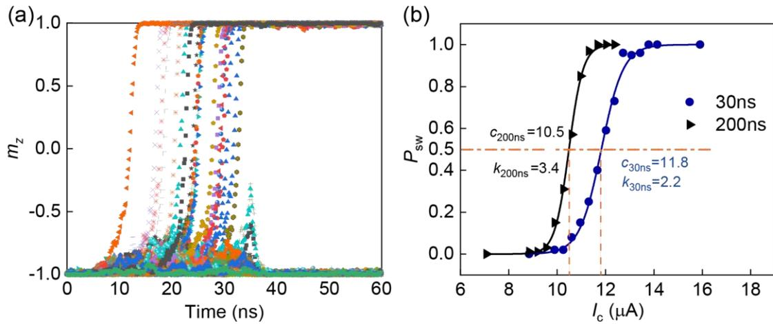
**Figure 5.** (a) The switching trajectories of 100 independent runs at  $I_c = 11.3 \mu A$  and 30 ns pulse width. The initial state is  $m_z = -1$ . The final state with  $m_z = 1$  indicates successful magnetization switching. (b) Illustration of  $k$  and  $c$  at different pulse widths.
