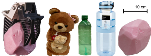
Fig. 8. From left to right: gripper grasping Styrofoam object, teddy bear, bottle for localization tests, bottle for grasping tests, Styrofoam object for baseline. Objects depicted at relative scale to each other.
