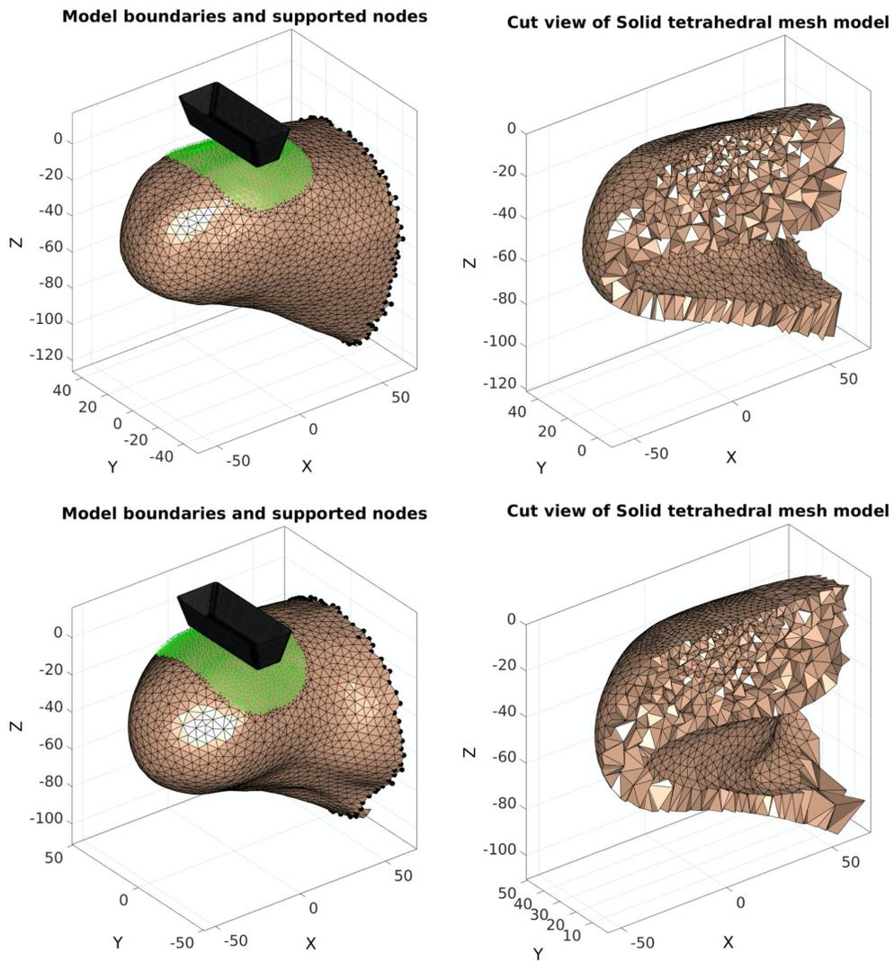
Figure 4: FE meshes of the anatomically accurate local computational model created from surfaces of bones and skin segmented from the MRI data. This allows for simulation of the ultrasound indentation. (Top) Subject 2, leg 1; (Bottom) Subject 2, leg 2.
