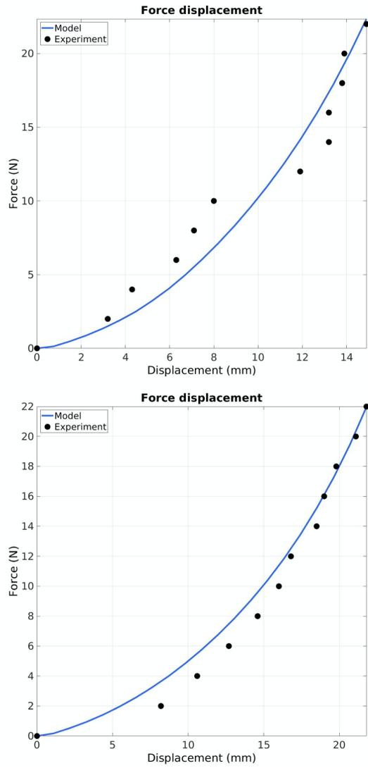
Figure 10: FEA results showing force-displacement curves from the raw data and the resulting curve fit from inverse FEA. (Top) Subject 1, indentation point 1; (Bottom) Subject 1, indentation point 2.
