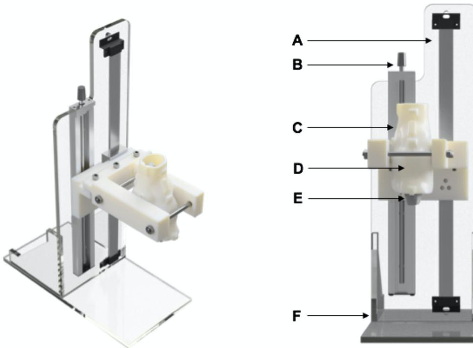
Figure 2: CAD rendering of ultrasound indentation setup. A Linear guide. B Knob to manually drive movement of the probe vertically for an indentation experiment. C Custom shell that mounts the ultrasound probe to the rest of the system. D Force sensor (located inside of shell, and mounted to the ultrasound probe). E Ultrasound probe. F Acrylic frame.
