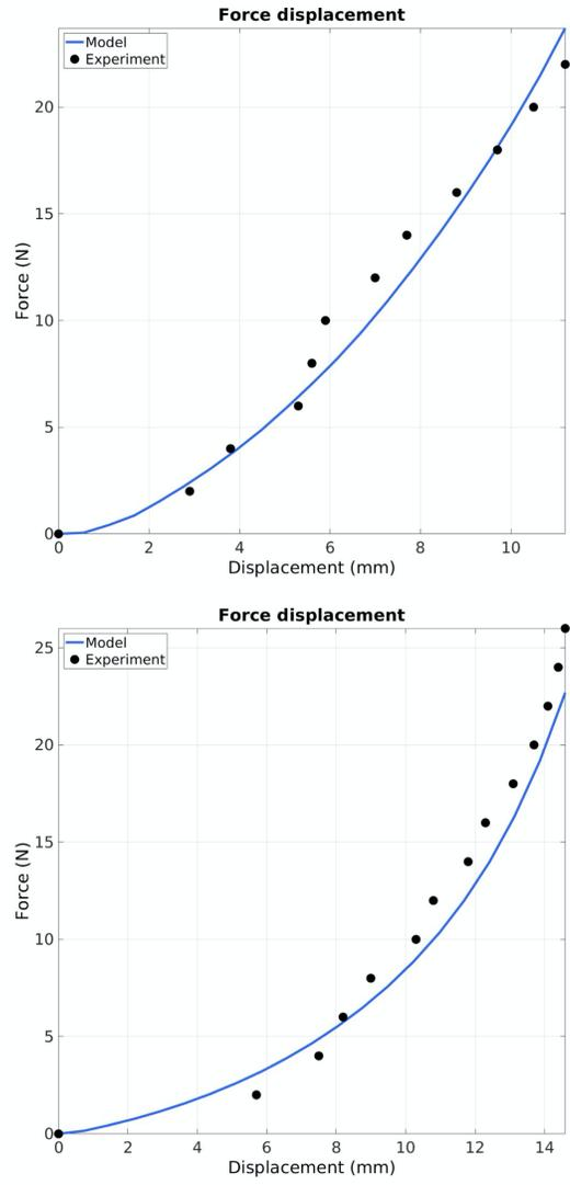
Figure 11: FEA results showing force-displacement curves from the raw data and the resulting curve fit from inverse FEA. (Top) Subject 2, leg 1; (Bottom) Subject 2, leg 2.
