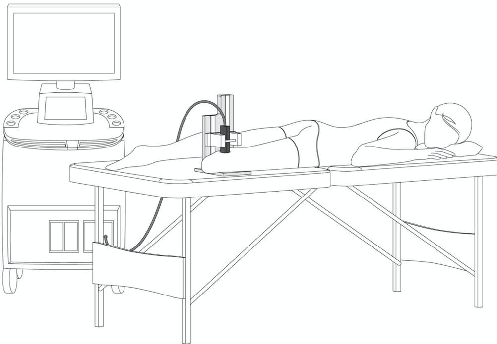
Figure 1: *Schematic showing overall indentation setup and patient positioning for experiments.*
