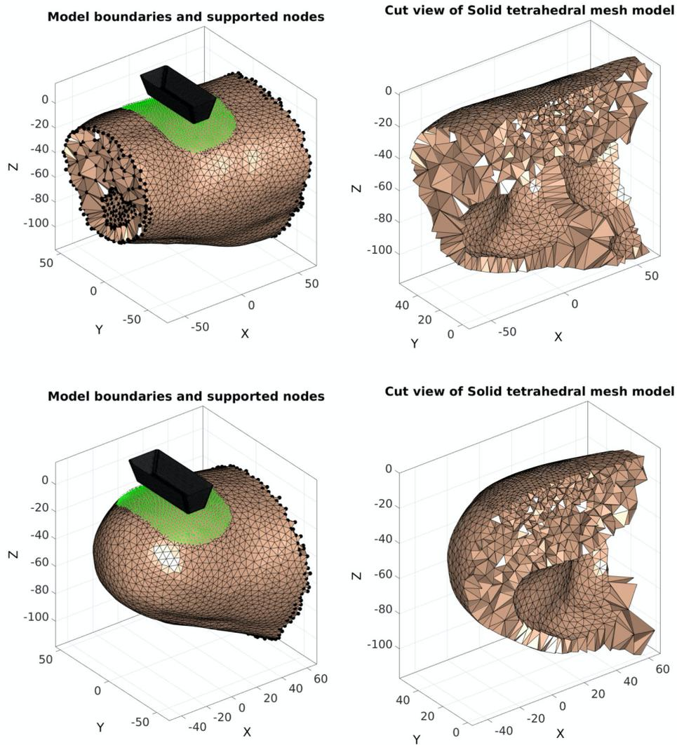
Figure 3: FE meshes of the anatomically accurate local computational model created from surfaces of bones and skin segmented from the MRI data. This allows for simulation of the ultrasound indentation. (Top) Subject 1, indentation point 1; (Bottom) Subject 1, indentation point 2.
