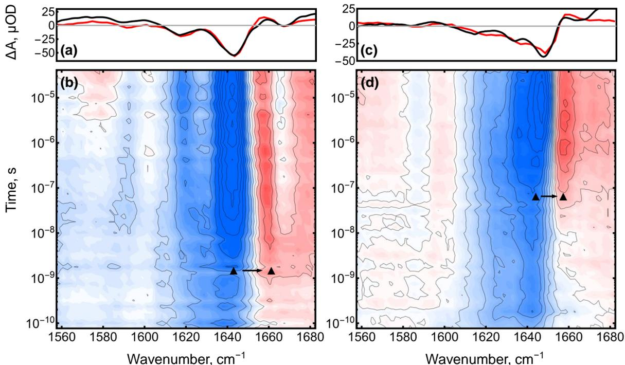
FIG. 4. IR spectroscopic analysis of PUMA (a,b) and NOXA (c,d) in complex with MCL-1. (a,c) Steady-state *cis*-to-*trans* difference spectrum (black) and the last kinetic trace at 42  $\mu$ s (red). (b,d) Transient *cis*-to-*trans* difference spectra as a function of pump-probe delay time. The triangles mark the blue shift of the amide I band from  $\approx 1640$   $\text{cm}^{-1}$  to  $\approx 1660$   $\text{cm}^{-1}$ .
