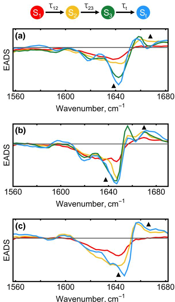
FIG. 6. Evolution associated difference spectra (EADS) of photo-perturbed (a) MCL-1/PUMA, (b) MCL-1/BIM (adapted from previous study<sup>32</sup>), and (c) MCL-1/NOXA. The triangles mark the blue shift of the amide I band from  $\approx 1640 \text{ cm}^{-1}$  to  $\approx 1660 \text{ cm}^{-1}$ .
