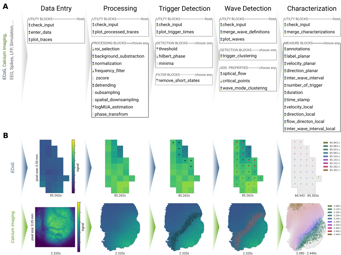
Figure 3. Progression of two datasets (ECoG in blue, wide-field calcium imaging in green) through the Cobrawap pipeline. A: The five successive stages contain collections of modular blocks in three different selection modes (fixed, choose one, choose any). The analysis path is adaptable for specific datasets and analyses by selecting and configuring the desired blocks (indicated by colored dots for the datasets). B: The intermediate results after each stage are visualized for the two datasets as color-coded signals on the electrode/pixel grid covering most of the right hemisphere of the mouse brain (up=anterior, right=lateral; ECoG: 4.95 \times 2.75 mm, calcium imaging: 5 \times 5 mm). From left to right: raw data, post-processed signal, detected upward transitions (black markers), grouped wavefronts (red markers) with the optical flow (arrows), and quantification of the linear flow alignment within the waves (i.e., planarity).
