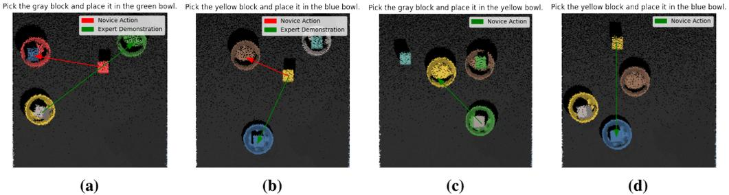
**Figure 3:** Example of learning how to recover thanks to on-policy data collection. The figures (a) and (b) show demonstrations for failure states, i.e., in (a) the block to be picked is already in another bowl, and in (b) there is already a block in the blue bowl. Such demonstrations of failure states are collected only in the interactive case. Figures (c) and (d) show that the novice can learn to recover from such failure states.
