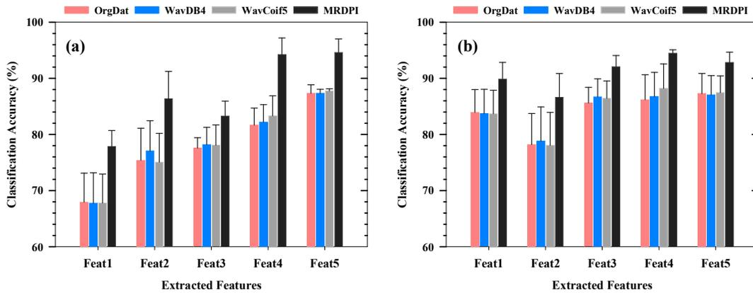
**Fig. 4:** Average motion intent decoding accuracy when the MRDPI is applied to process multi-class EMG signals compared with using signals processed via WaveletDB (WavDB4), WaveletCoif (WavCoif5), and the Original Data (OrgDat) across feature sets for (a) LDA and (b) RF. \* *Using In-house Custom Dataset.*
