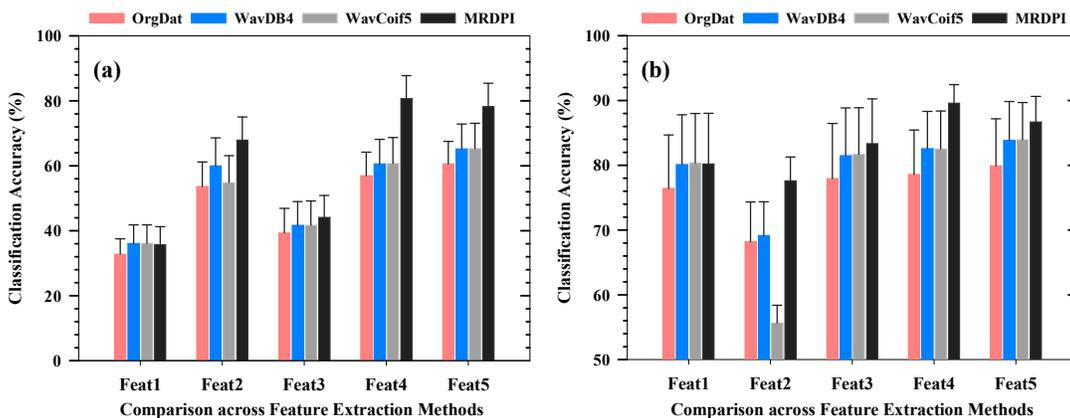
**Fig. 5:** Average motion intent decoding accuracy when the MRDPI is applied to process multi-class EMG signals compared with using signals processed via WaveletDB (WavDB4), WaveletCoif (WavCoif5), and the Original Data (OrgDat) across feature sets for (a) LDA and (b) RF. \* *Using Public NinaPro Dataset.*
