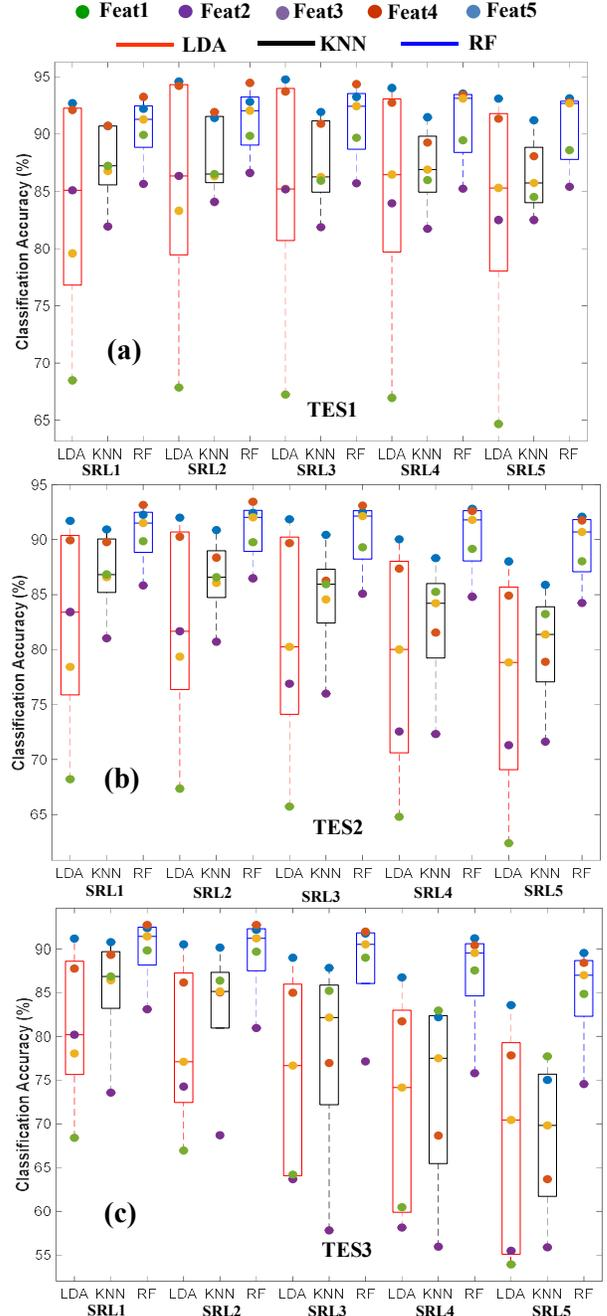
**Fig. 3:** Average motion intent decoding accuracy based on denoised and reconstructed EMG signals via the MRDPI across SRL (SRL1-SRL5) and TES: (a) TES1 (b) TES2 and (c) TES3. The results were averaged across motion classes and subjects for each feature-classifier combination.
