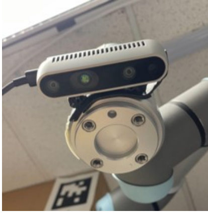
Fig. 3. Intel Real sense D435i mounted on the end-effector for taking measurement
