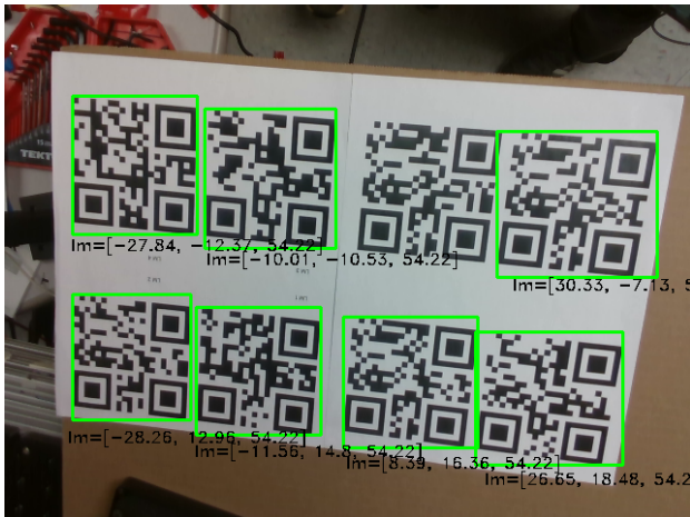
Fig. 4. Results of data association and distance measurement (measurement values in centimeters)
