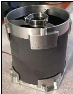
Figure 4. The SPARCS telescope is RC design, with a carbon fibre tube coated in anti-reflection paint.
