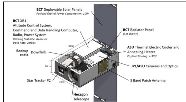
Figure 6. SPARCS payload integrated to the BCT SPACECRAFT. Communications provided via S-band. Ground stations are provided by KSAT-lite. Solar panels deploy in space. Two star trackers plus low-jitter reaction wheels provide pointing stability to  $< 6''$ .
