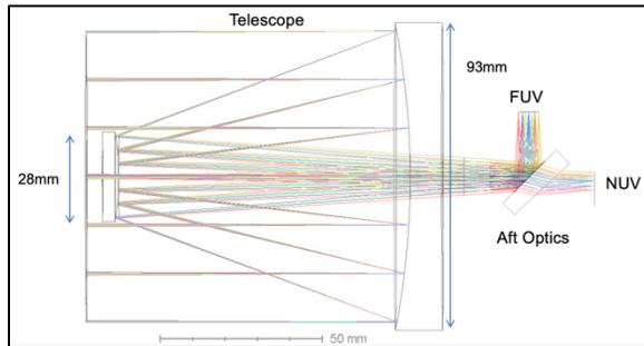
Figure 3. SPARCS Optical Train. The Aft optics element hosts the dichroic, the NUV filter, and performs aberration correction.
