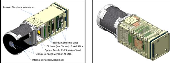
Figure 2. *Top:* Block diagram for the SPARCS Payload. The payload processor implements automatic exposure control, while the payload temperature controller manages the thermal system. *Bottom:* The SPARCS payload is very compact, and fits within 3U of the spacecraft. It has a dedicated radiator (not shown), isolated from the spacecraft. Materials have been chosen for their low outgassing characteristics, to prevent optical contamination. Venting paths allow payload outgassing to space.
