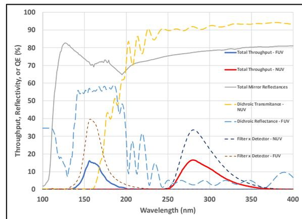
Figure 5. Component and system reflectivities, throughputs, or QE. SPARCS maximum throughput is ~15% in both bands, compared with GALEX's 3% maximum NUV throughput [10].
