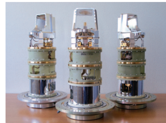
▲ Receivers for the ALMA telescope, made by NOVA based on technology partly developed at SRON.
