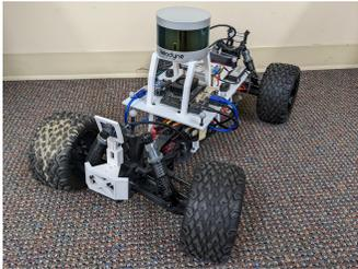
Fig. 2: Fully equipped ART vehicle platform
