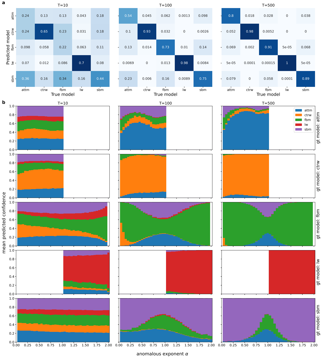
FIG. 8: Analysis of the classification behaviour. (a) Confusion matrices for different trajectory lengths. The entries indicate the relative frequency of model predictions (row) given a ground truth model (column). The matrices are obtained from Multi-SWAG predictions on a total of 10^5 test trajectories for each length.
