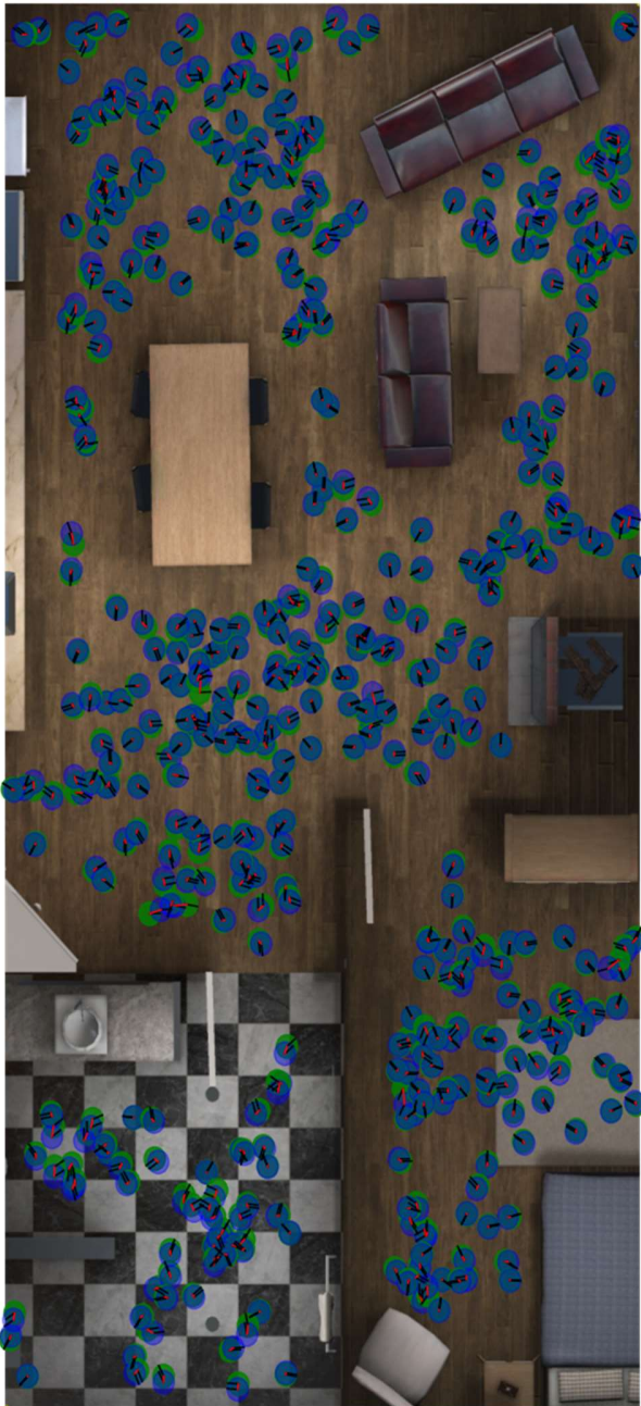
Figure 5. Ground truth (green) and predicted (blue) poses for each sample in the Cabin test set. Black lines show sample orientation, red lines show distance error.
