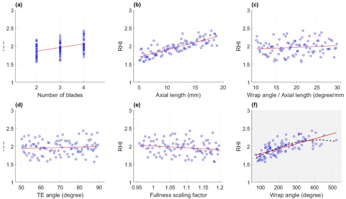
Figure S1. Sensitivity of the relative hemolysis index, RHI, in Exploration 2. (a)-(e) RHI plotted against input variables with 1st-order fit plotted in solid red. (f) RHI plotted against wrap angle (reconstructed by multiplying axial length and wrap angle / axial length ratio) with 2nd-order fit shown in dashed line.
