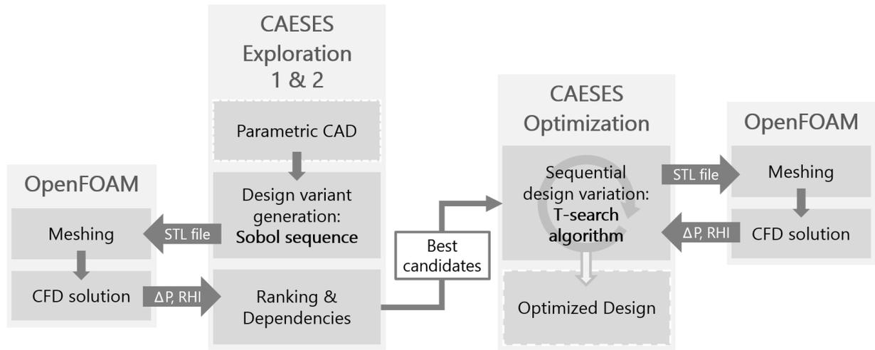
Figure 3. Schematic depiction of the optimization process and communication between the CAESES and OpenFOAM modules.
