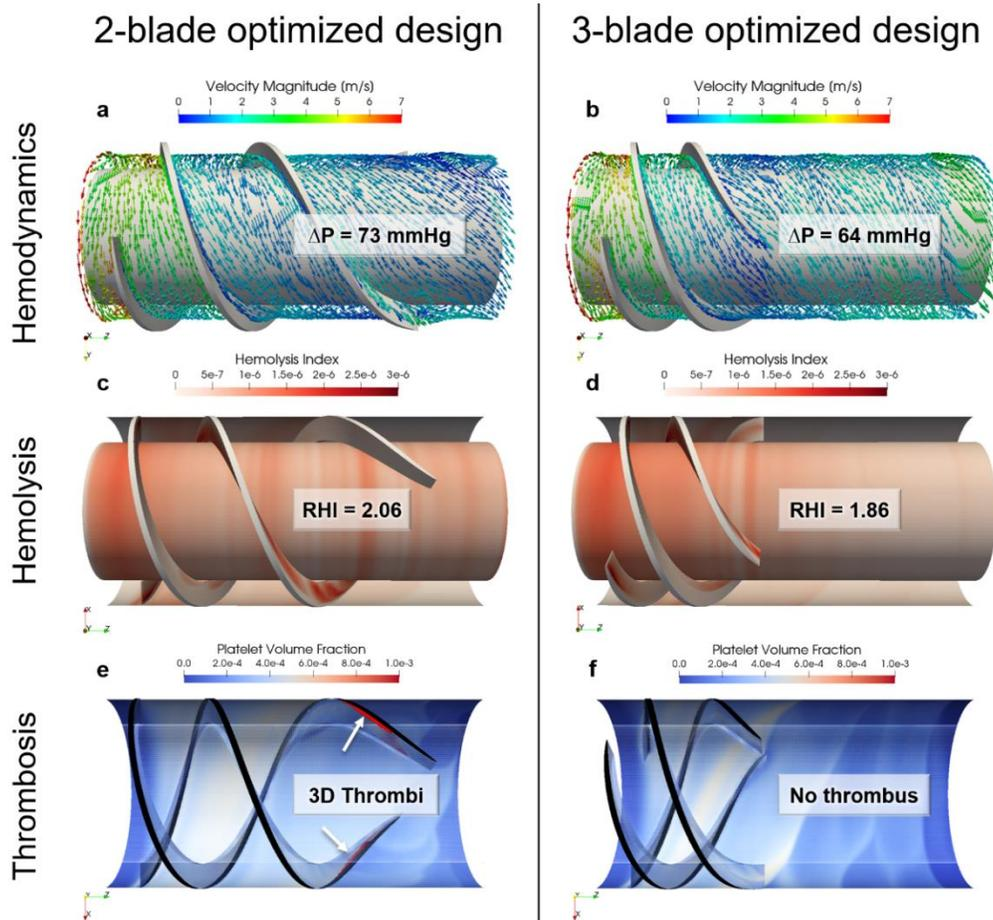
Figure 7. Comparison of optimized 2-blade and 3-blade designs. Flow is from left to right. (a, b) Velocity vectors presented at mid span. (c, d) RHI shown on blood contacting surfaces. (e, f) Thrombosis simulation results shown at 30 min of simulation time. The deposited platelet volume fraction is shown on blade and shroud surfaces; threshold volume fraction for 3D thrombus visualization is  $> 0.1$ . The hub surface remained free of thrombus in both cases.
