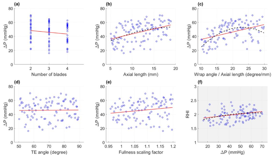
Figure 5. In Exploration 2, the wrap angle input parameter was replaced with the ratio of wrap angle to axial length, constrained to the favorable range identified from Exploration 1. (a)-(e) Pressure recovery,  $\Delta P$ , plotted against input variables with 1<sup>st</sup>-order fit plotted in solid red and 2<sup>nd</sup>-order fit shown in dashed line. (f) The relative hemolysis index, RHI, plotted against  $\Delta P$  reveals that pressure recovery came at the cost of increased hemolysis.
