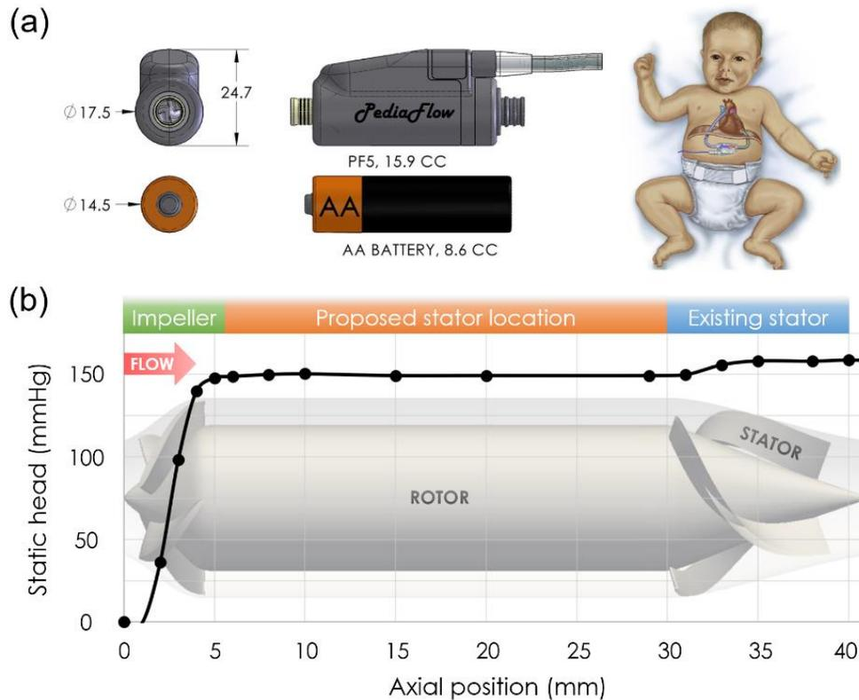
Figure 1. (a) The fifth-generation PediaFlow VAD dimensions (mm) compared to an AA-battery, designed for children from birth to 2 years of age. (b) Static head produced by PF5 at 1.5 LPM and 16,000 RPM plotted along the axial position. The image of the current PF5 rotor and stator is overlaid on the plot. The proposed mid-stator location is indicated in orange.
