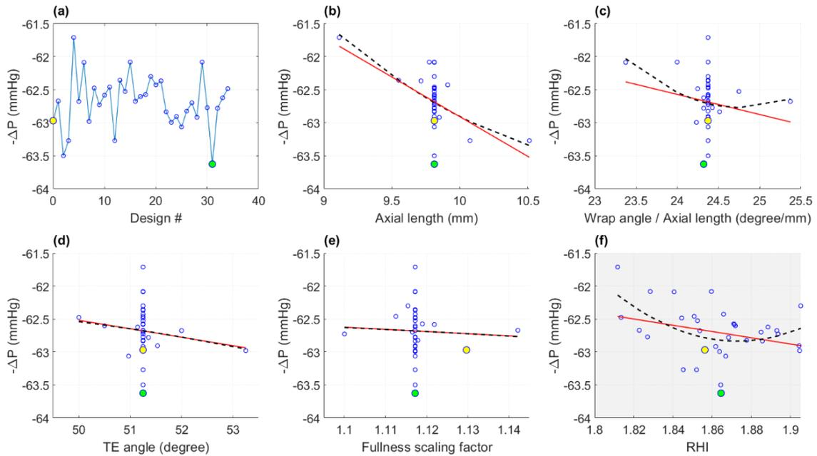
Figure S3. Local optimization of the best 3-blade candidate using the T-search algorithm. The initial design point is highlighted in yellow, and the final (optimized) design is highlighted in green. (a) The evolution of the objective function with consecutive design variations. (b)-(e) The objective function plotted against the input variables. (f) The gain in pressure recovery came at the cost of increased hemolysis, RHI.
