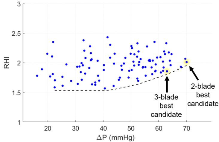
Figure 6. The relative hemolysis index, RHI, plotted against  $\Delta P$  from Exploration 2. Dashed line traces the outer envelope of designs with the lowest RHI for given  $\Delta P$ . Arrows point to the two best candidates selected for further local optimization.
