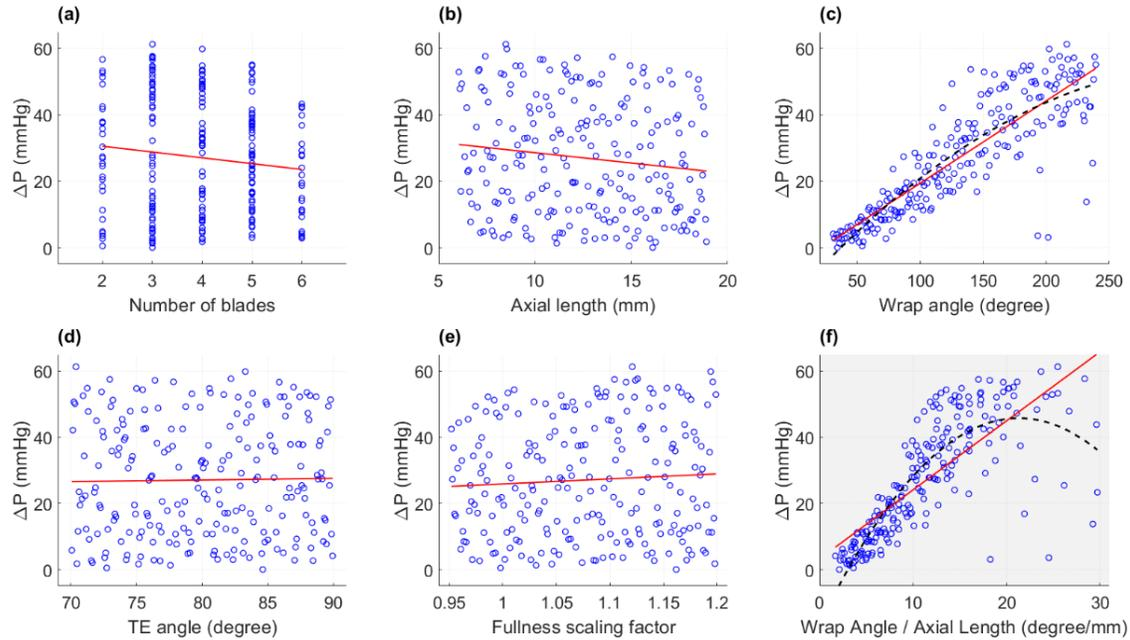
Figure 4. Results of Exploration 1. (a)-(e) Pressure recovery,  $\Delta P$ , plotted against input variables with 1<sup>st</sup>-order fit plotted in solid red and 2<sup>nd</sup>-order fit shown in dashed line. Only designs that produced pressure rise are shown. (f) Pressure recovery plotted against the ratio of wrap angle to axial length showed a sharp increase in the range between 10 and 30 degree/mm.
