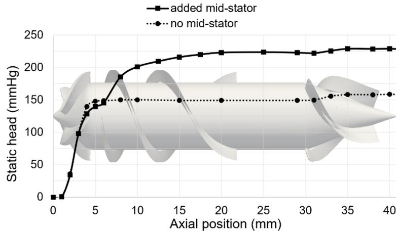
Figure 8. Performance of the optimized 2-blade design in the PF5 pump at 1.5 LPM and 16,000 RPM compared to the baseline. The image of PF5 with added mid-stator is overlaid on the plot to match the axial position; original PF5 not shown.
