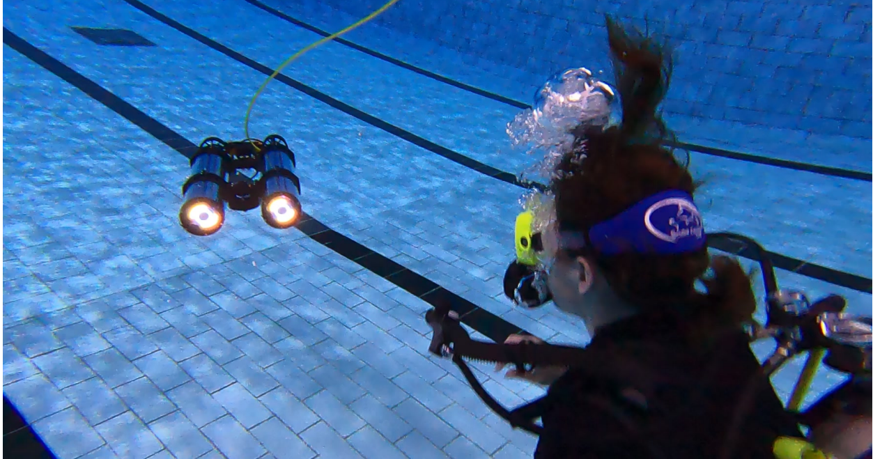
Figure 1: The LoCO AUV informs a diver that it is ready to follow them, using the active luceme FollowYou L .
