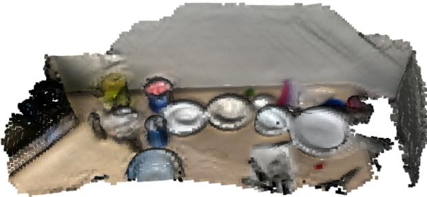
Figure 3. Point cloud generated from HoloLens 2 data using Open3D [27].
