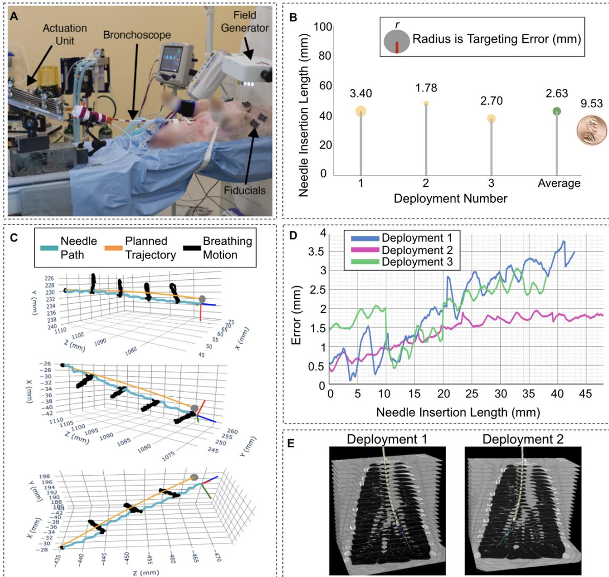
**Fig. 4: In vivo porcine lung results.** (A) The in vivo experimental setup. (B) Results for all system deployments with needle steer length on the y-axis, steer number on the x-axis, and a circle with radius equal to the targeting error. The penny is for scale. (C) Planned and tracked needle trajectories. (D) Magnitude of the trajectory error for each deployment. (E) Visualization of the deployments shown within slices of the CT scan of the anatomy.
