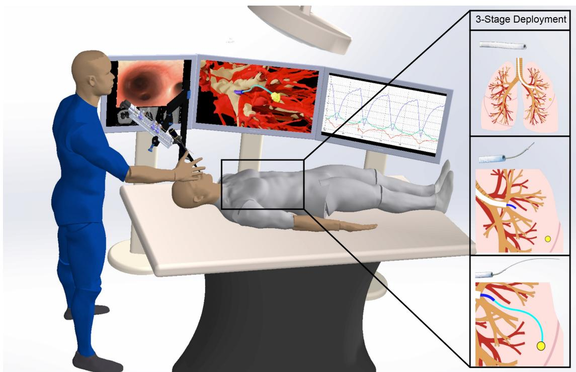
**Fig. 1: Overview of the semi-autonomous medical robot’s three stages in the lungs.** Stage 1 consists of a physician manually navigating a traditional bronchoscope through the airways. Stage 2 consists of a physician teleoperating the aiming device. Stage 3 consists of autonomous needle deployment through the parenchyma to the nodule while accounting for respiratory motion and avoiding anatomical obstacles such as clinically-significant vasculature, bronchi, and the visceral pleural boundary.
