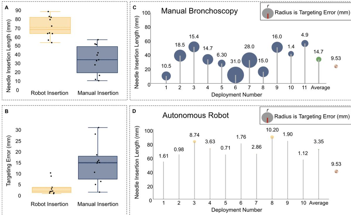
**Fig. 5: Results from the comparison experiments between the manual bronchoscopy and the proposed robotic system.** (A) Deployment lengths. (B) Targeting errors. (C) Results from the manual bronchoscopy deployments. (D) Results from the robotic steerable needle deployments.
