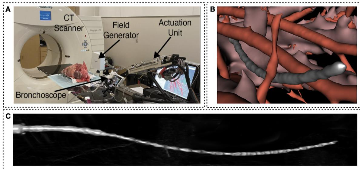
**Fig. 6: Capabilities of the flexible steerable needle.** (A) The ex vivo experimental setup. (B) Segmentation of the steerable needle following deployment in ex vivo lungs. (C) The 3D rendering of the steerable needle corresponding to the segmentations.
