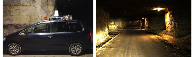
Fig. 20: Kvarntorp dataset collected within an underground mine. A car with a roof-mounted radar was driven 1235 m at a speed of 10km/h in a loop to an endpoint close to the starting location. The vertical passages are feature-poor and challenging to localize within.
