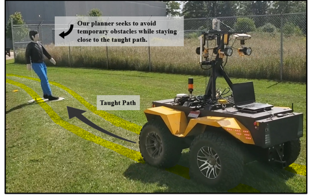
Fig. 1. We present an architecture for locally avoiding unmapped obstacles along a reference path by extending sample-based motion planners to encourage trajectories with characteristics that best exploit prior path knowledge. Our system is validated on a Grizzly robot in real-world scenarios.
