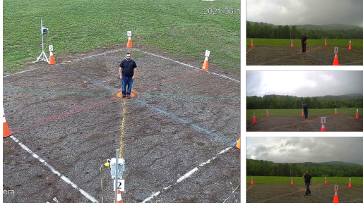
Figure 3: Close-range station example from BGC1. The image on the left is a single frame collected from an elevated surveillance camera. The images on the right are frames from the standing and walking portions of the subject collection viewed from ground-level cameras.
