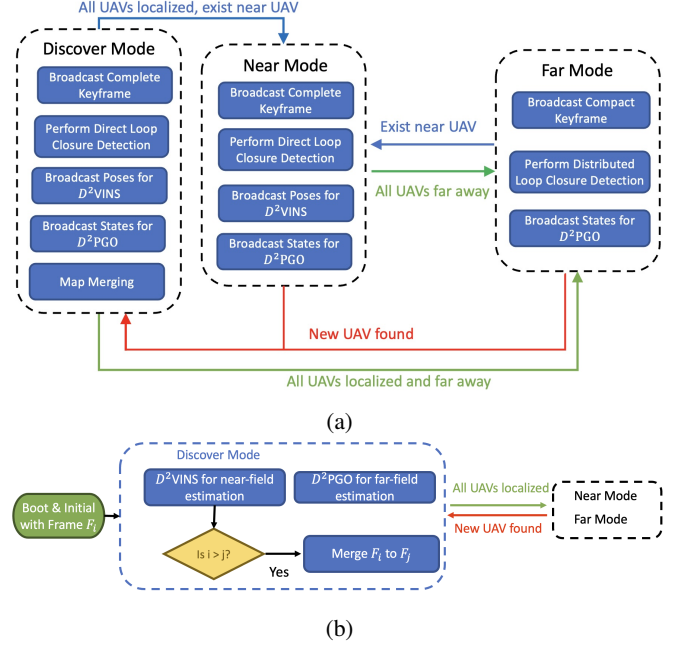
Fig. 4: a) A state machine governing D^2 SLAM's communication modes begins in discover mode. In this initial phase, each UAV broadcasts its complete keyframe to support rapid initialization and transmits data essential for D^2 VINS. Once UAVs have successfully initialized their relative states, D^2 SLAM transitions to either near or far mode, depending on their estimated relative positions. The system can fluidly alternate between near and far modes in response to changes in UAV positioning. Importantly, if a new UAV enters the system, typically seen during the initialization phase, D^2 SLAM reverts to discover mode to incorporate this new member. b) Map merging occurs during the discover mode, as shown in the flow charts. If near or far-field state estimation identifies other UAVs, the UAV with the higher index transfers its map state to the UAV with the lower index.
