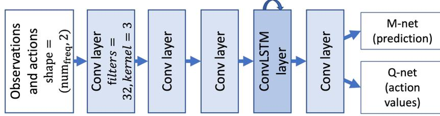
Figure 3: ConvLSTM-DAN architecture with Q and M outputs. The ConvLSTM is convolutional in frequency and recurrent in time.
