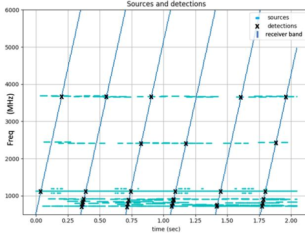
Figure 1: A partially observed RF environment with sequential scan for control, which misses the short signal bursts at 1.2GHz. Plot: time(sec) vs frequency(MHz); cyan: signals; dark blue: sampled bands; black x marks: detected signals.
