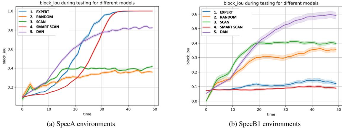
Figure 6: Comparison: hand-coded controllers expecting SpecA vs. ConvLSTM-DAN only trained in SpecA environments: (a) testing in SpecA; (b) testing in SpecB1. Hand-coded performance degrades significantly more than DAN when environments deviate from expected/training spec. Plot: Block IoU vs. time; 100 sampled test environments per spec.
