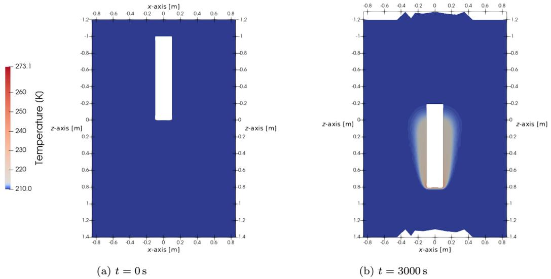
Figure 7: Temperature-controlled displacement of the probe over time due to close-contact melting. On the left, the initial state with the tip at  $z = 0$  m is pictured. On the right, we show the computed position and temperature distribution after 3000 s.
