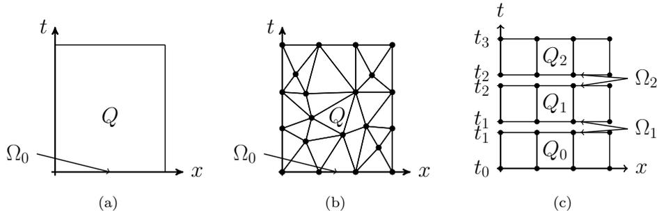
Figure 3: (a) Space-time domain with discretizations according to (b) the C-SST and (c) the D-PST approach.
