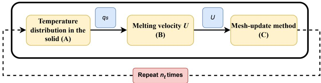
Figure 2: Overview of the scale-coupled computational approach at each time step. The macro-scale temperature distribution **(A)** around the heat source is computed via space-time finite elements. The melting velocity **(B)** is then retrieved according to the micro-scale model in Sections 2.1 and 2.2, where the latter requires the numerical heat flux  $q_s$  at the phase interface. Finally we apply the velocity  $U$  to the mesh movement **(C)**.
