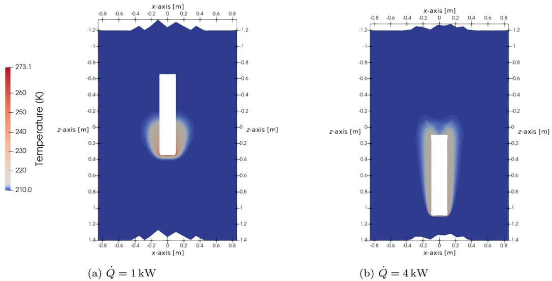
Figure 8: Power-controlled displacement of the probe over time due to close-contact melting. We show the computed position and temperature distribution after 3000 s for two values of heat-flow rate.
