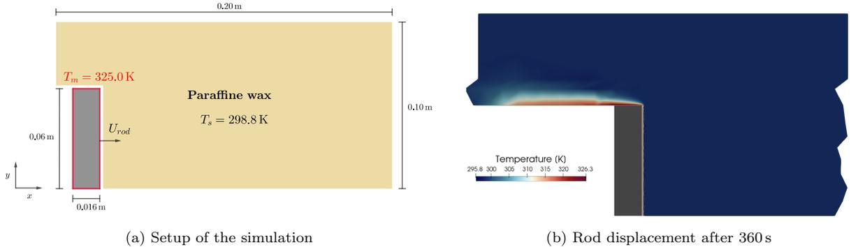
Figure 11: 2D hot-wire cutting simulation. A hot copper wire is pressed against a solid block of wax, which has the initial temperature  $T_s = 298.8$  K (a). After 360 s the rod has cut halfway through the block (b).
