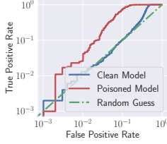
Figure 2: Membership inference against the airplane class of CIFAR-10 dataset. The poisoning budget is set as b_{\text{poison}} = 10\% \times |\mathcal{D}_{\text{clean}}| . The AUC score, i.e., the area under the ROC curve, is increased from 0.6917 to 0.9255, indicating that our dirty-label poisoning attack is effective.
