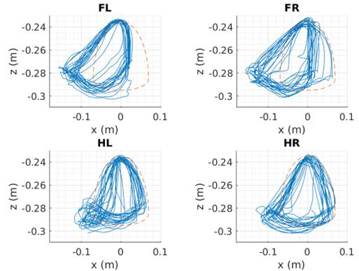
Fig. 5: Leg frame foot  $XZ$  trajectories for a deployed policy locomoting at 0.8 m/s with dynamically added mass. Significant modulations can be seen to the sample task space trajectory represented by the dotted line. Notably, the amplitude for the front feet shifts the trajectory to lie mostly behind the hip, produces a continuum of more natural gaits that are less rigid, more efficient, more robust, and have lower frequency.
