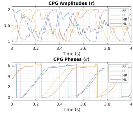
Fig. 4: CPG states for 1 second of a deployed policy locomoting at 0.8 m/s. An approximate trot gait can be observed, with faster swing time ( $0 \leq \theta \leq \pi$ ) than stance time. Coordination between the amplitude and phase variables can be seen, noticeably increasing amplitude in stance phase to push backward and propel the quadruped forward.
