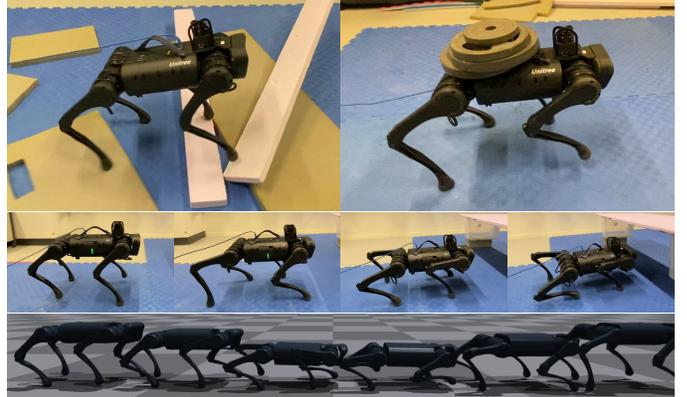
Fig. 1: Quadruped locomotion with CPG-RL. **Top**: crossing uneven terrain (left), and walking at 0.8 m/s with a 13.75 kg load representing 115% of the nominal quadruped mass (right). **Bottom**: user-specified body height modulation to crawl underneath a ledge, both experiment and simulation.
