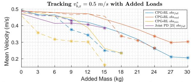
Fig. 6: Sim-to-sim mean velocity for command  $v_{b,x}^* = 0.5$  m/s under increasing added loads. The dashed lines represent the same method/observation trained without any noise in Isaac Gym. The \*s represent when performance is not guaranteed: the robot sometimes falls down, or cannot make consistent forward progress.
