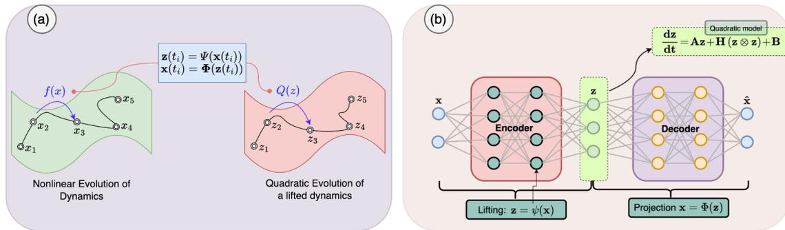
Figure 1.1: The figure illustrates that nonlinear dynamical systems can be written as quadratic dynamical systems in an appropriate finite-dimensional lifted coordinate system. In the right plot, we depict a neural network architecture to learn a lifted coordinate system that has the desired quadratic embeddings.
