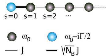
Figure 8. **Illustration of the right-side semi-infinite chain model.** Here, a trap is located on site  $s = 0$  and a hopping defect is connecting sites  $s = 0$  and  $s = 1$ .
