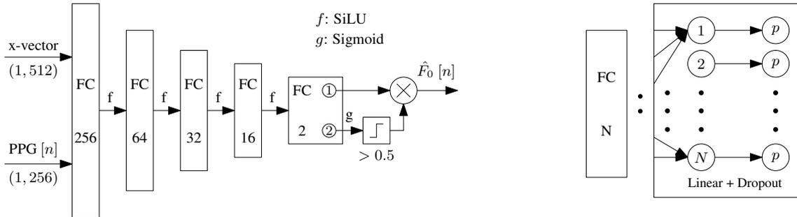
Figure 2: (a) Architecture of our proposed neural network. The numbers below the expression "FC" denote the number of neurons in each layer. "FC" denotes a fully connected layer. The circles with numbers 1, 2 in the last layer denote the output of  $n$ th neuron in that layer (after dropout if applicable).
