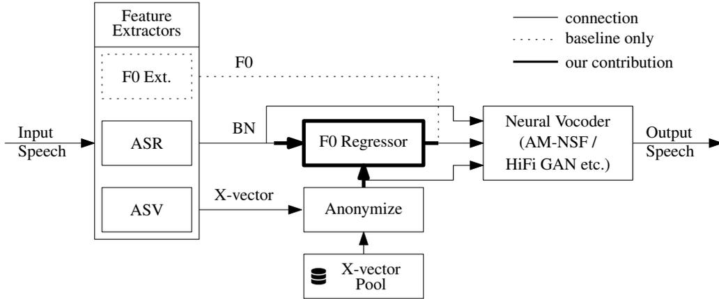
Figure 1: Signal flow diagrams of the baselines B1.a (if neural vocoder is an AM-NSF), B1.b (if neural vocoder is NSF with GAN) and joint-hifigan (if neural vocoder is the original HiFi-GAN) together how our contribution "F0 regressor" is integrated.
