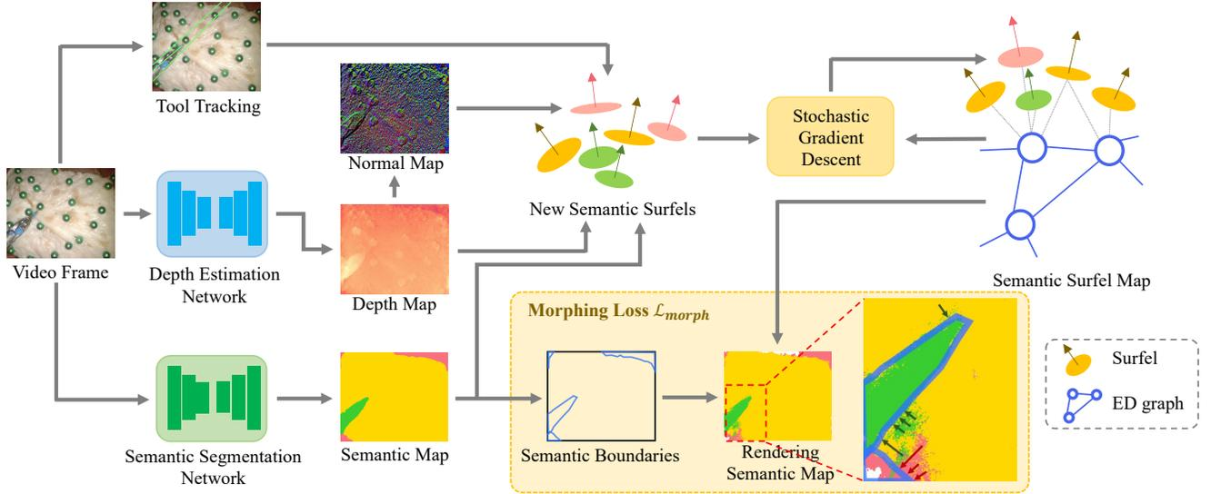
Fig. 2. **Overview of the proposed framework.** The depth, semantics, and tool poses are extracted from the input video frame. The transformations of ED nodes are optimized to match the observations under several constraints, including a semantics-based morphing loss. The optimization is implemented using stochastic gradient descent [36] with PyTorch’s automatic differentiation. Surfel position and normal updates are then controlled by the ED nodes.
