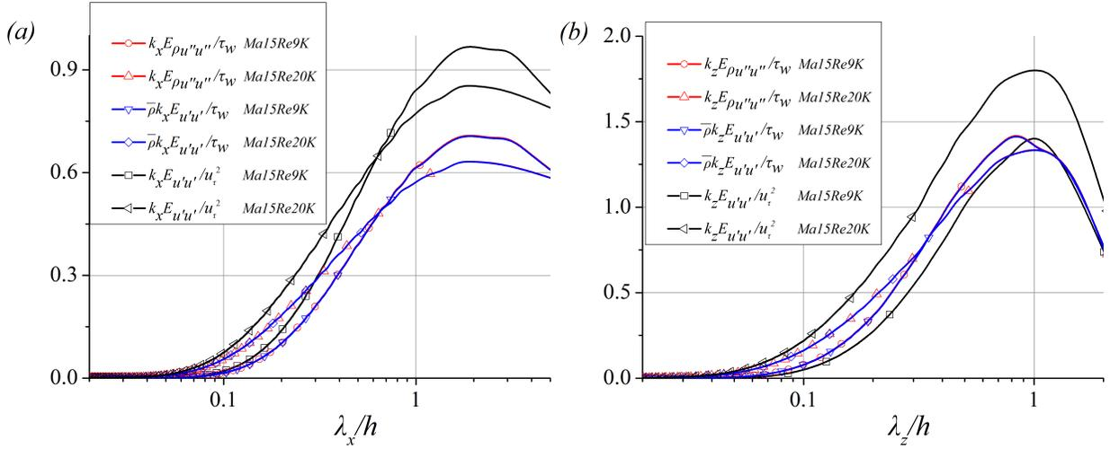
Figure 7. Streamwise (a) and spanwise (b) premultiplied spectra of the streamwise velocity fluctuations for Ma15Re9K and Ma15Re20K at  $y = 0.2h$  with different density-weighted approaches and without density weighting.
