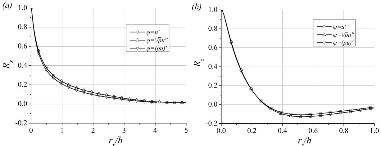
Figure 4. Streamwise (a) and spanwise (b) two-point correlations of  $u'$ ,  $\sqrt{\rho}u''$ , and  $(\rho u)'$  for the case Ma15Re20K at  $y/h = 0.2$ .
