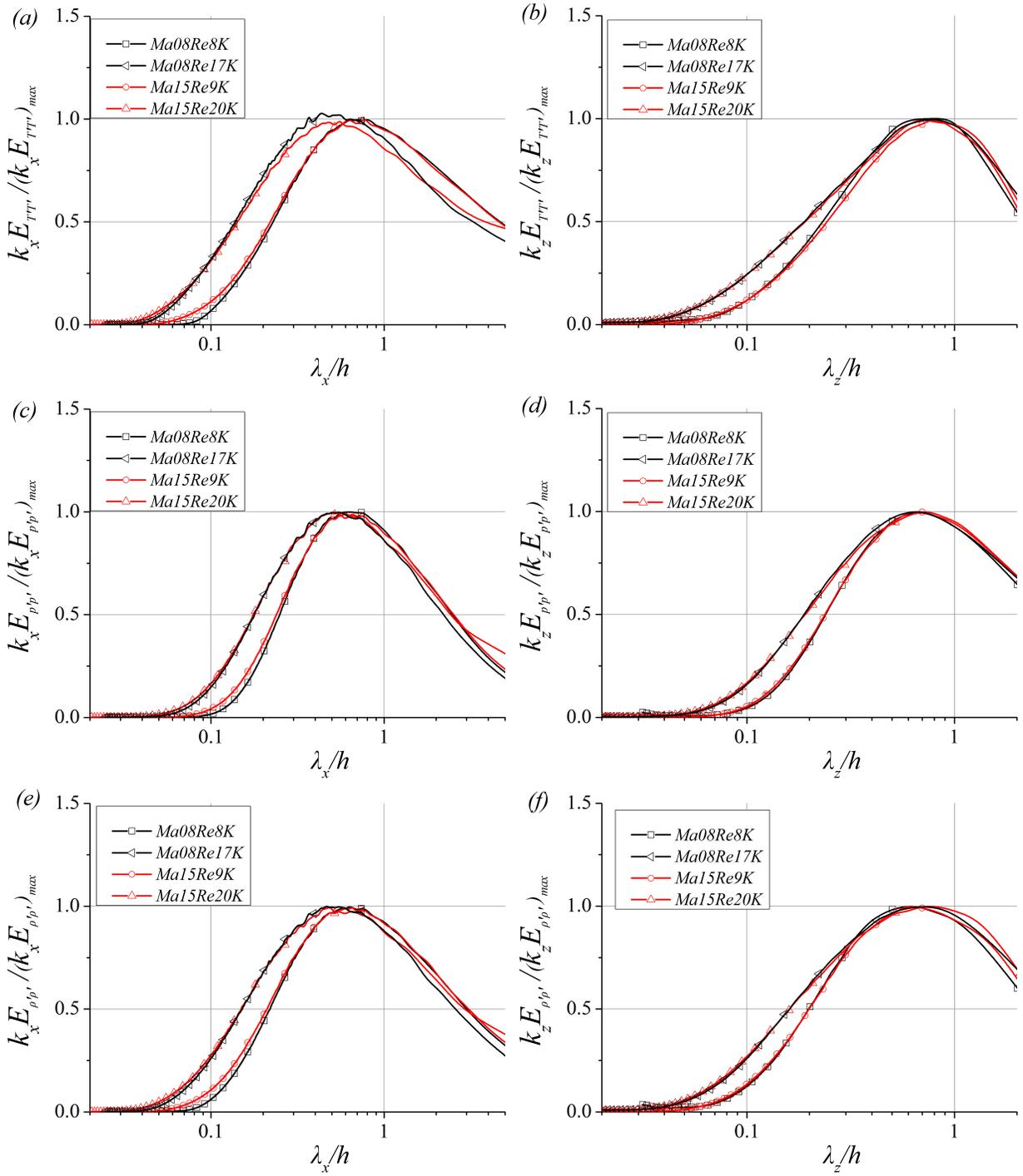
Figure 6. Streamwise (a,c,e) and spanwise (b,d,f) pre-multiplied one-dimensional spectra of  $T'$  (a,b),  $p'$  (c,d), and  $\rho'$  (e,f) for all compressible cases at  $y/h = 0.2$ . All the spectra are normalized by their maximum values.
