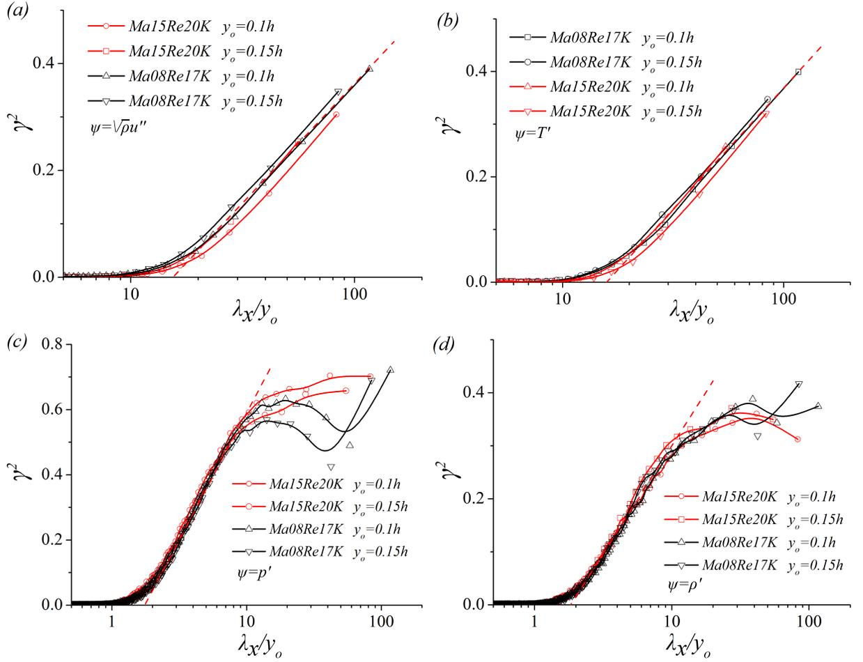
Figure 9. Variations of  $\gamma^2$  as functions of  $\lambda_x/y_o$  at two selected wall-normal heights, i.e.,  $y_o = 0.1h$  and  $y_o = 0.15h$ , for  $\psi = \sqrt{\rho}u''$  (a),  $T'$  (b),  $p'$  (c), and  $\rho'$  (d), respectively. The dashed lines in the subfigures denote the logarithmic growth Eq. (4).
