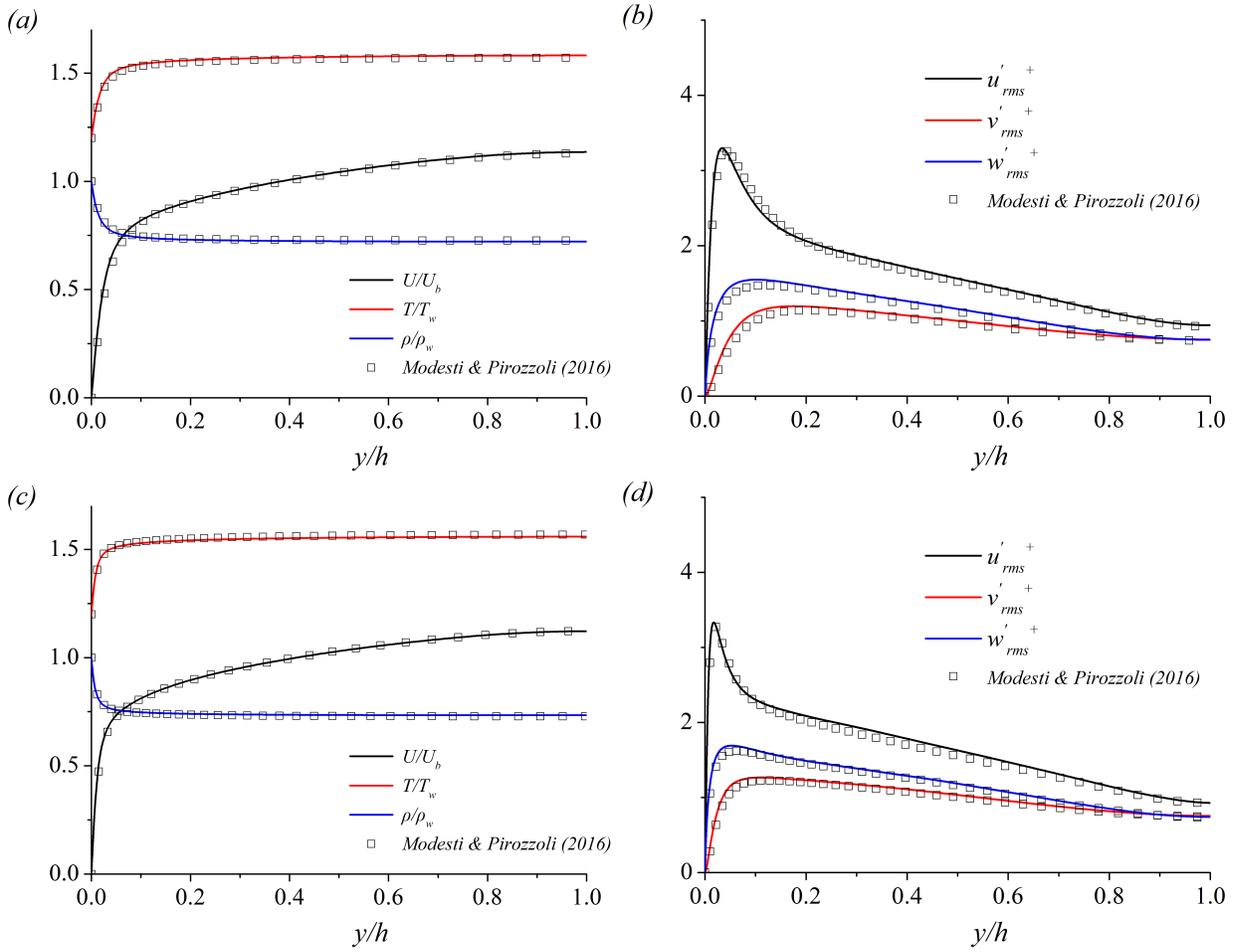
Figure 2. Profiles of mean streamwise velocity, mean temperature, and mean density for the cases Ma15Re9K (a) and Ma15Re21K (c); profiles of the root-mean-square of the velocity fluctuation for the cases Ma15Re9K (b) and Ma15Re21K (d). The profiles of  $T/T_w$  are shifted upward by  $\Delta(T/T_w) = 0.2$  for better comparison.
