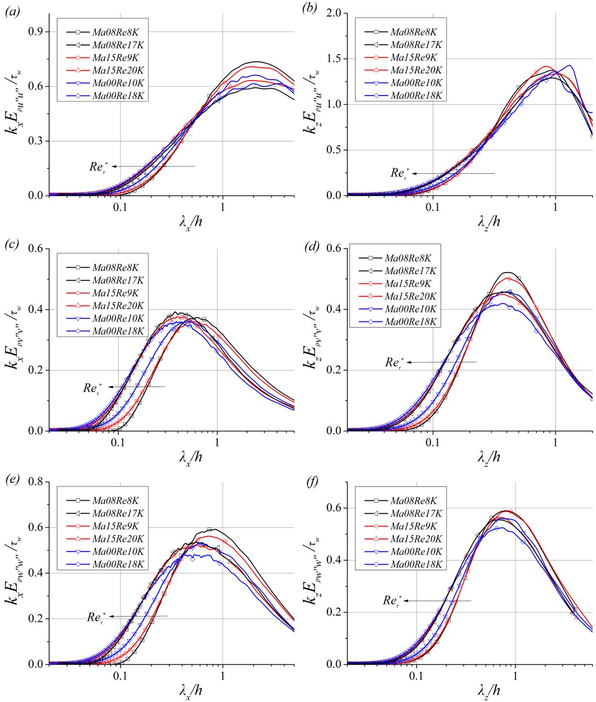
Figure 5. Streamwise (a,c,e) and spanwise (b,d,f) premultiplied one-dimensional spectra of  $\sqrt{\rho}u''$  (a,b),  $\sqrt{\rho}v''$  (c,d), and  $\sqrt{\rho}w''$  (e,f) for all cases at  $y/h = 0.2$ .
