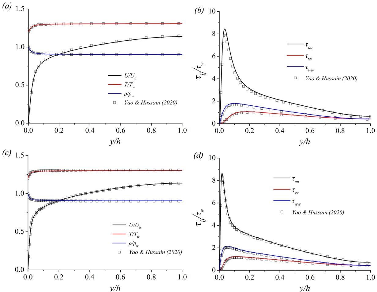
Figure 1. Profiles of mean streamwise velocity, mean temperature, and mean density for the cases Ma08Re8K (a) and Ma08Re17K (c); profiles of the Reynolds stress for the cases Ma08Re8K (b) and Ma08Re17K (d). The profiles of  $T/T_w$  are shifted upward by  $\Delta(T/T_w) = 0.2$  for better comparison.
