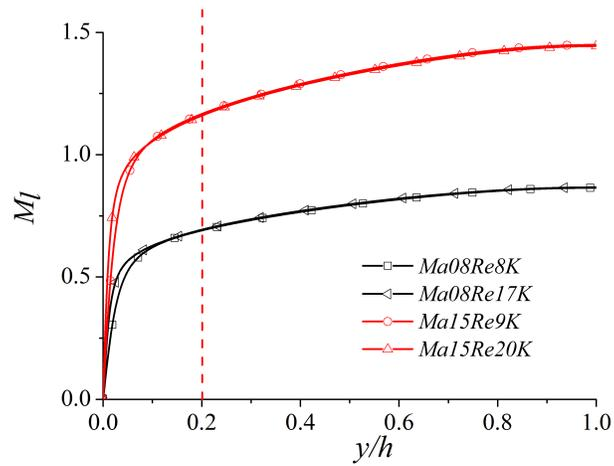
Figure 3. Profiles of mean local Mach number for all compressible cases. The red dashed line indicates  $y = 0.2h$ , i.e., the wall-normal position for investigation in the present study.
