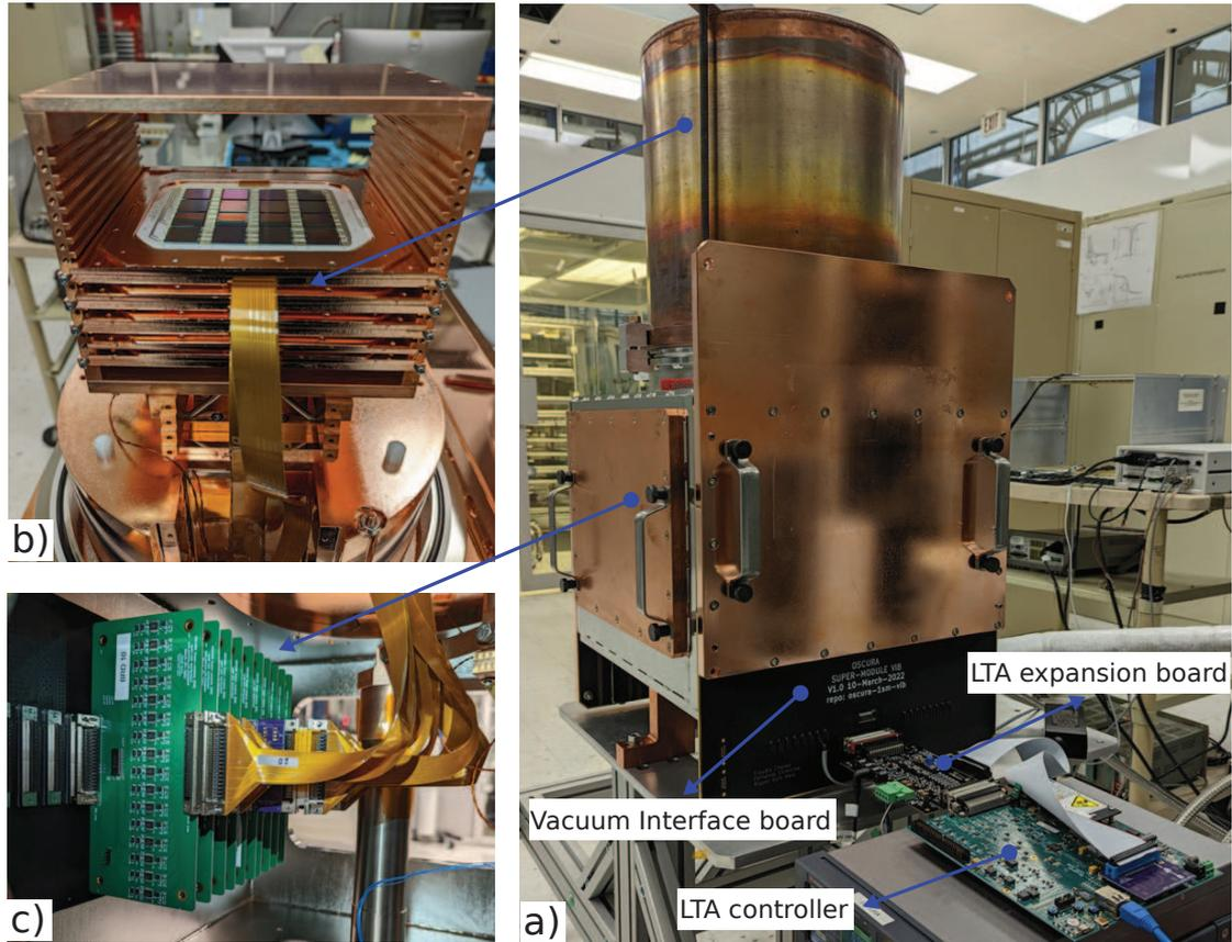
**Figure 2:** a) Photograph of the exterior of the instrument: cylinder in the top holds the sensors, box in the bottom houses the frontend electronics; b) Copper box and copper trays holding the sensors and flex cables; c) frontend electronics connected to the vacuum interface board.
