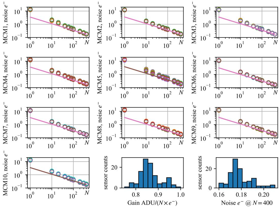
**Figure 7:** Noise in  $e^-$  as a function of the number of samples per pixel  $N$  for all the MCMs and channels. The two histograms at the right bottom show the gain and noise computed for  $N = 400$ .
