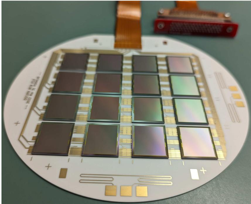
**Figure 3:** Photograph of a Multi-Chip Module (MCM): single layer ceramic substrate with 16 glued single-electron resolution Skipper-CCDs.
