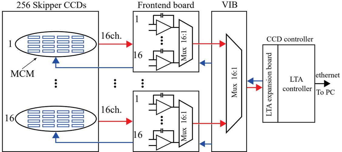
**Figure 1:** Block diagram of the multiplexed architecture capable of controlling and reading up to 256 Skipper-CCDs. Red lines indicate the path of video signals and blue lines illustrate the CCDs clock signals, bias voltages and frontend control signals.
