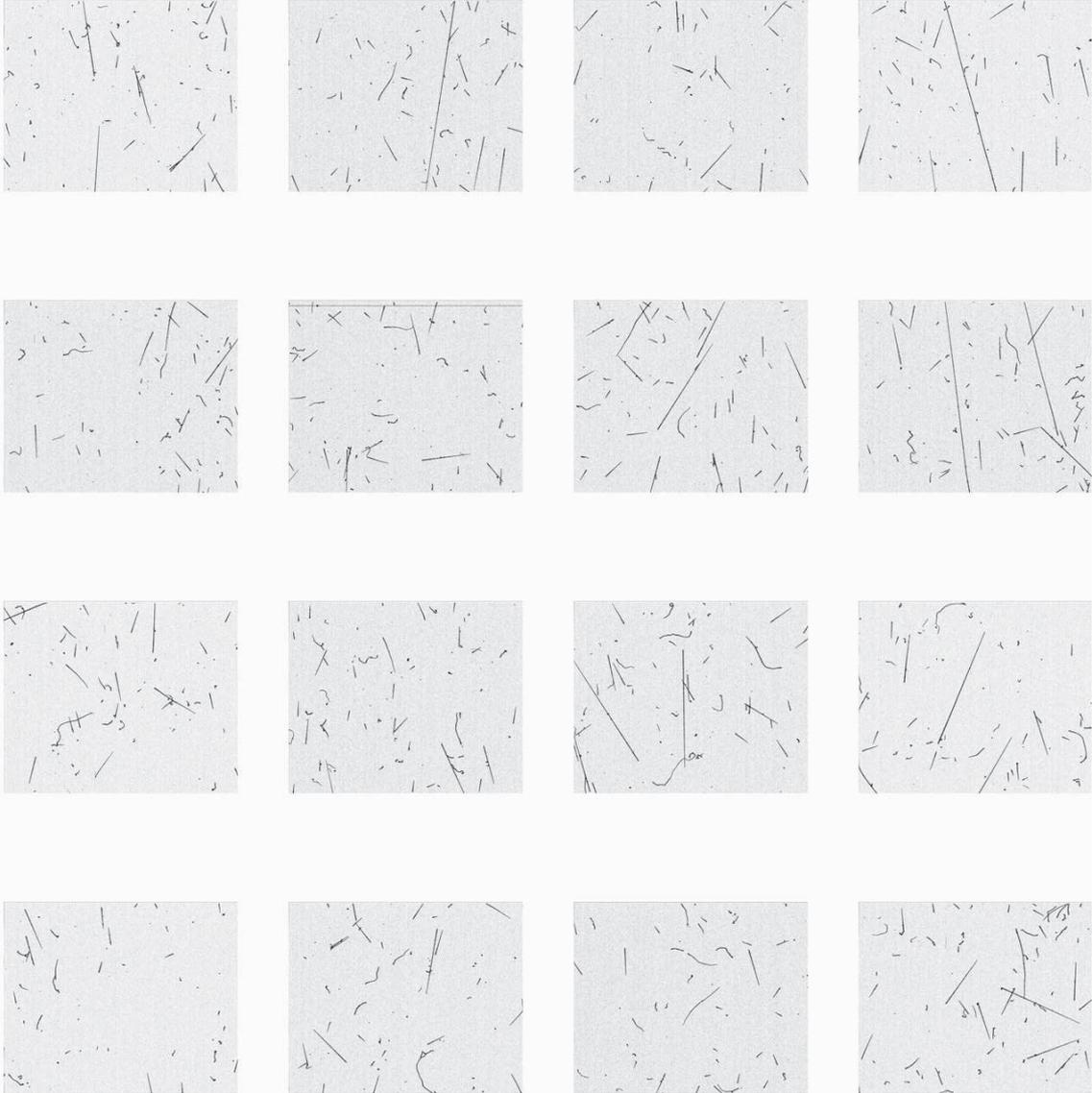
**Figure 5:** Full image of a single MCM with 16 sensors. Each sub-image corresponds to a 1.35 Mpix sensor and are separated by the space in the physical arrange. Muons crossing more than one sensor can be appreciated. The color scale in this image was inverted compared to Fig. 4.
