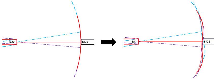
Fig. 1. Schematic diagram of how TTL-Wavefront distortion coupling occurs. (left) The ideal transmitted beam with the Jitter propagating into the telescope aperture of another spacecraft. (right) The propagation of the beam carrying wavefront errors. The truncated wavefront is transformed from the spherical wave(left) to the distorted one(right).
