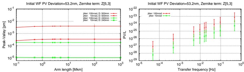
Fig. 6. (left) PV values relevant to the arm length from  $10^{-1}$  to  $10^3$  Mkm. (right) the calculated P/V/L values with the transfer frequency increasing.
