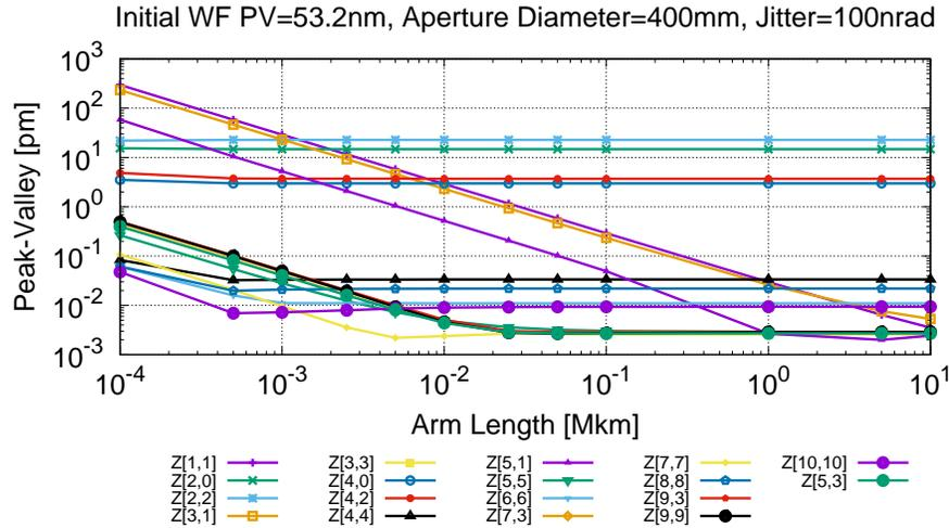
Fig. 3. At 100 nrad jitter, PV values of the wavefront error of distorted gaussian beam at the receiver after propagation, which are relevant to the different Zernikes. The initial wavefront error is constrained to 53.2 nm. The diameter of telescope aperture is 400 mm.
