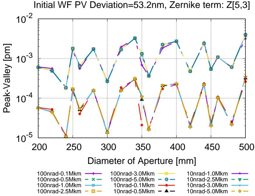
Fig. 5. At Zernike Z[5,3], PV values of the Wavefront error of propagated beam with the telescope aperture diameter increasing at the transmitter.
