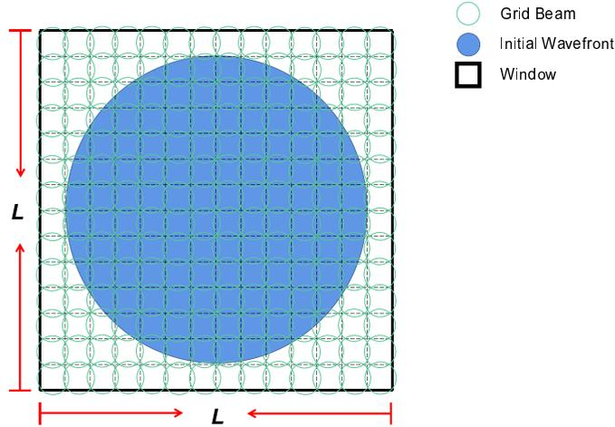
Fig. 7. A simple illustration of GBD method. The green one is fundamental grid Gaussian beam, which is arranged in window. The window in the graph is chosen to be square. The blue one is the wavefront to be decomposed.
