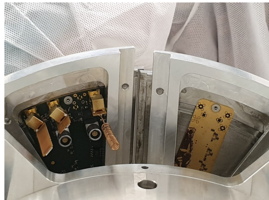
FIG. 11: Antennae for the wireless communication connected perpendicularly to the surface of the PCB.
