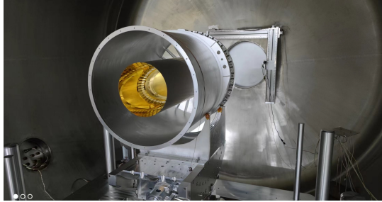
Fig. 19 Mirror sample of eXTP installed in the chamber of 100XF.
