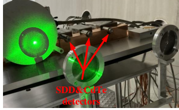
Fig. 13 Two SDDs and one CdTe are applied to monitor the X-ray beam during the test of a Micro-Slot-Optics telescope.
