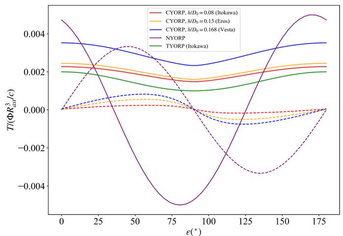
**Fig. 7.** Comparison between the CYORP, TYORP, and NYORP torques, which are shown in different colors. The solid curve denotes the spin component, and the dashed curve denotes the obliquity component.
