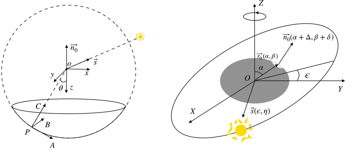
**Fig. 2.** Three coordinate systems in this paper: Coordinate system  $oxyz$  for calculating the illuminated domain in the crater,  $PABC$  for calculating the effective recoil force of an arbitrary surface element, and  $OXYZ$  for averaging the YORP torque over the spin and orbital motion.
