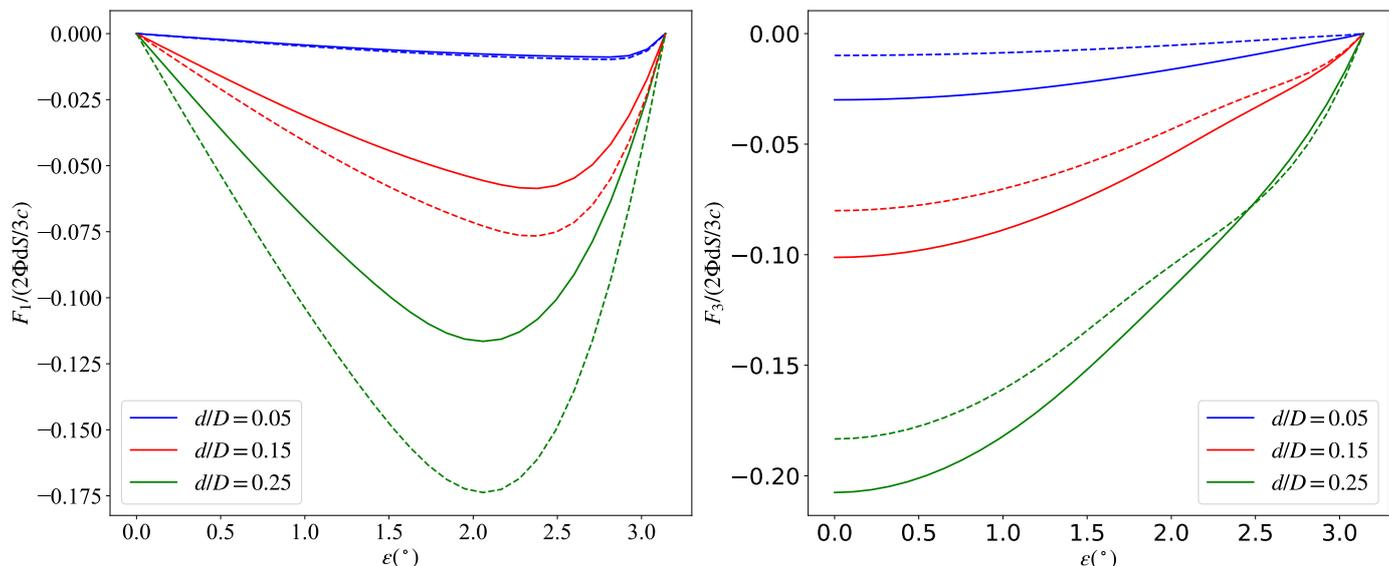
**Fig. 5.** Recoil forces for craters with different  $h/D_0$ . The results considering the self-heating effect are shown by solid lines, and the results obtained without the self-heating effect are shown by dashed lines. The left panel denotes the tangential component of the recoil force, and the right panel denotes the normal component.
