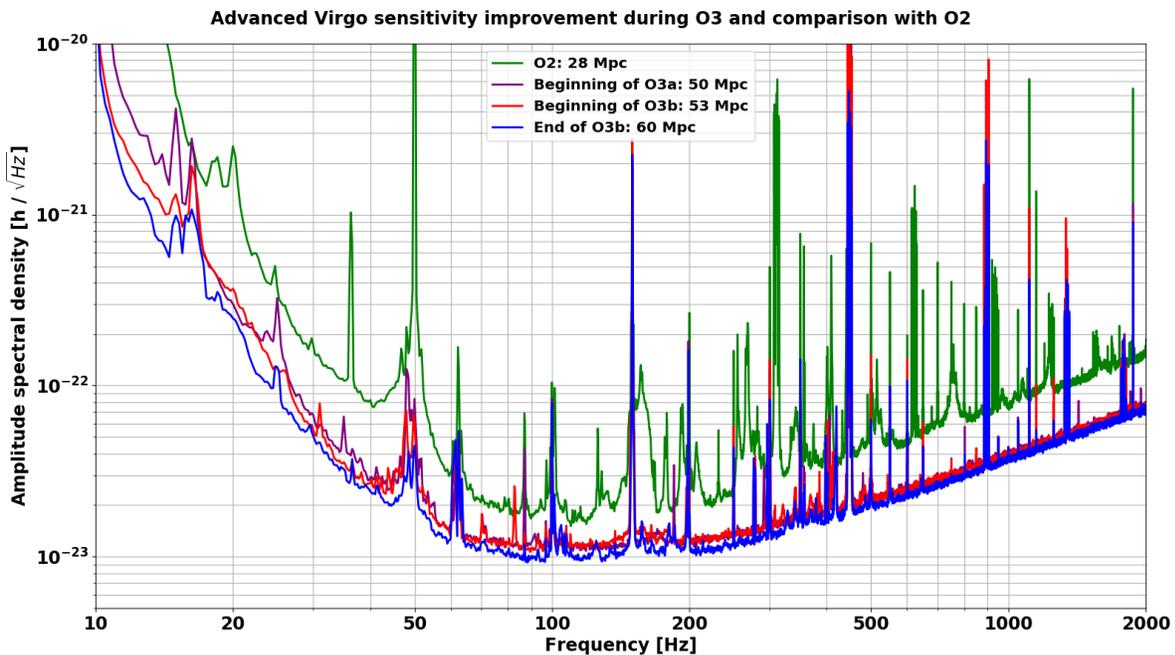
**Figure 8.** Comparison between four sensitivity curves of the AdV detector: during O2 (green trace), at the beginning of O3a (purple), at the beginning of O3b (red) and at the end of O3b (blue). The caption provides the corresponding estimated BNS ranges.
