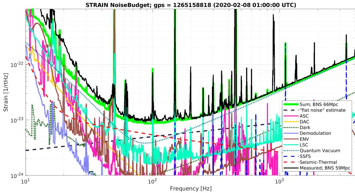
**Figure 6.** Snapshot of the AdV O3 noise budget generated at a time of near best sensitivity of the detector (February 8<sup>th</sup>, 2020). The different noise sources shown are described in the text. The green line (BNS range: 66 Mpc) represents the sum of these noises: it can be compared to the measured total noise shown in black (BNS range: 59 Mpc).
