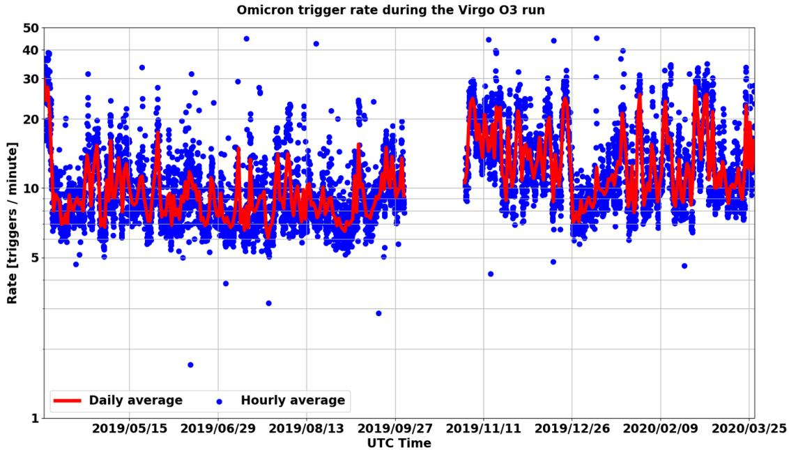
**Figure 14.** Virgo glitch rate, using `Omicron` triggers, for the final O3 dataset (Science segments that have not been CAT1-vetoed). The blue dots are averages over one hour while the red curve shows the corresponding daily moving average. The gap in between O3a and O3b corresponds to the 1-month commissioning break.
