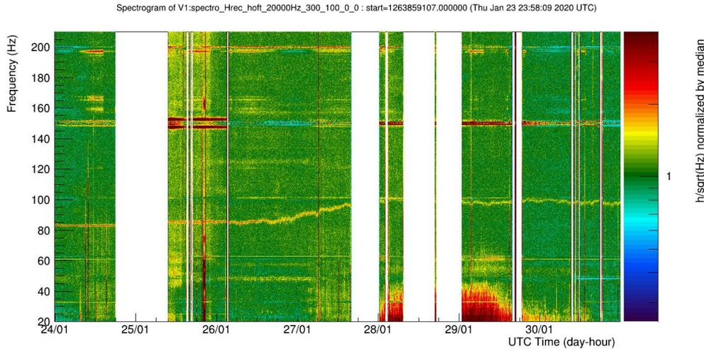
**Figure 18.** A typical 7-day spectrogram of the  $h(t)$  channel, generated by the `Spectro` tool [16] and allowing the monitoring of a wandering spectral line whose main frequency was first stable around 83 Hz before increasing up to around 100 Hz in about a day.
