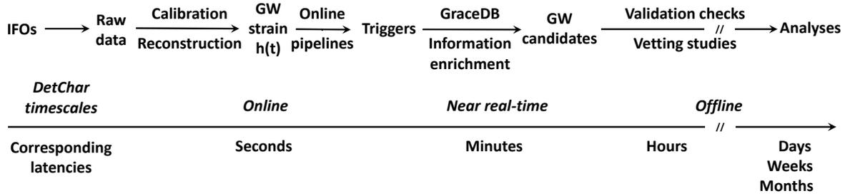
**Figure 5.** Dataflow from the interferometers (labeled "IFOs" on the left) to the offline validation of GW candidates and the completion of the final dataset (right). It focuses on the generation and the vetting of the public alerts that are a key product of the LIGO-Virgo observing runs. It shows the three main timescales at which the Virgo DetChar group operates: online, near real-time and offline (see text for details).
