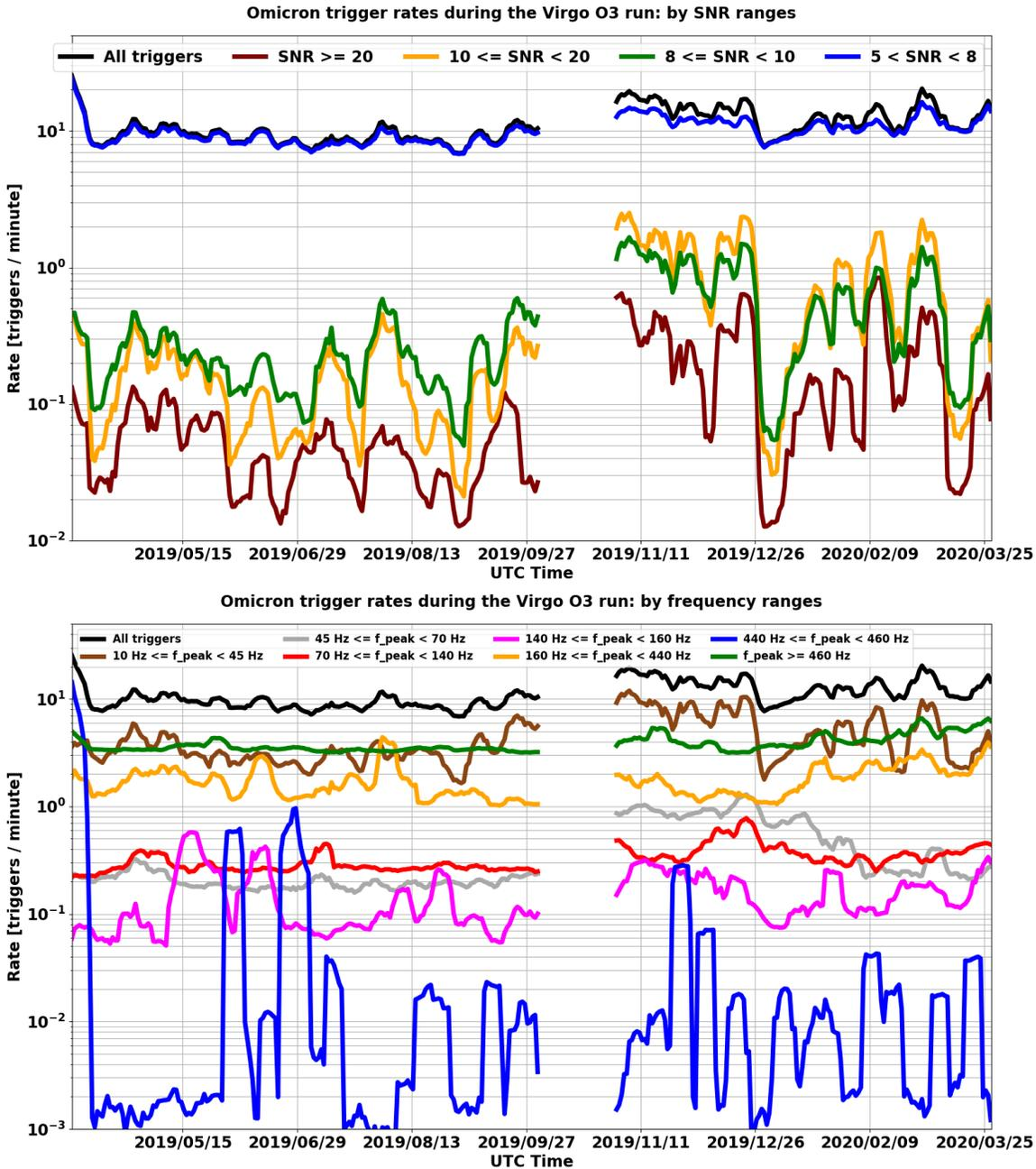
**Figure 15.** Glitch rates (daily moving average) using Omicron triggers during the O3 run for Virgo. The gap in between O3a and O3b corresponds to the 1-month commissioning break. The top plot breaks the glitch rate into SNR ranges, while the bottom one categorizes it in terms of frequency ranges for the glitch peak frequency.
