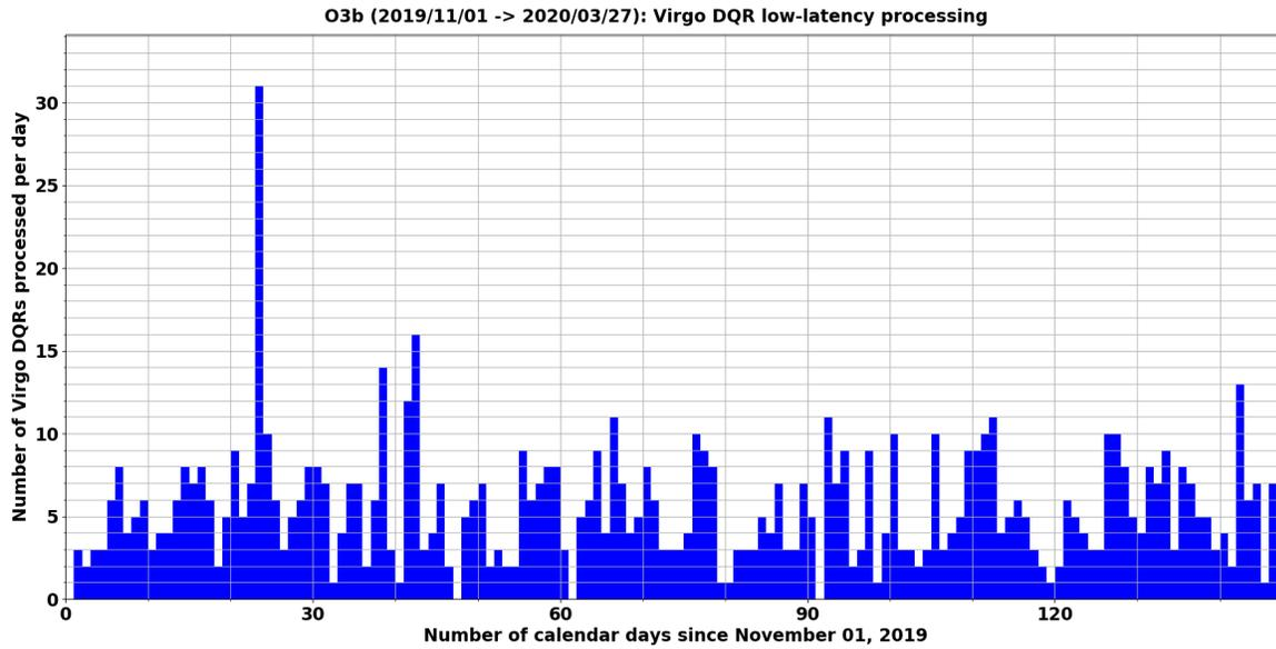
**Figure 12.** Number of Virgo DQRs automatically processed per day during the O3b run. The peak of 31 entries corresponds to November 24<sup>th</sup>, 2019 when there was a transient problem with the Virgo  $h(t)$  reconstruction: that generated several online triggers, finally including S191124be that passed the public alert threshold and was promptly retracted.
