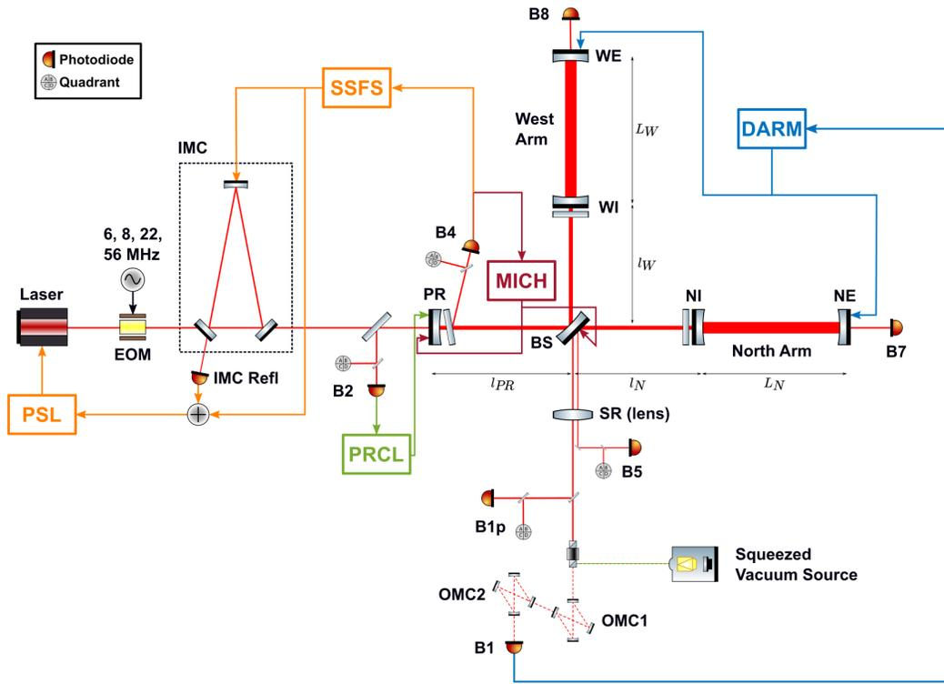
**Figure 2.** Schematics of the AdV configuration during the O3 run (not to scale), showing optics, photodiodes and quadrant photodiodes, such as the main components of the global feedback system used to steer the detector. The suspended optical benches introduced in the text are not represented here. This figure is taken from [31].
