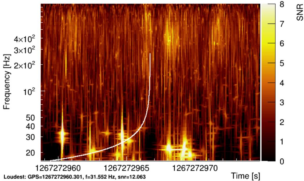
**Figure 13.** Omicron spectrogram around the time of the S200303ba trigger. The search template time-frequency track (solid line) overlaps with low-frequency scattering-light glitches (yellow color) caused by bad weather.
