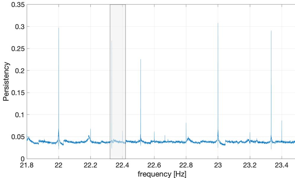
**Figure 17.** Plot of line *persistence* over the frequency band 20 Hz to 30 Hz. The grey box identifies the frequency range covered by a narrow-band search of CW signals from the Vela pulsar in O3a data. The line at 23.333 Hz, which contributed to produce a candidate in the search is clearly visible. In fact, several other lines belonging to the 1 Hz *comb*, both at integer frequencies and shifted by 0.333 Hz, and to a weaker 0.2 Hz-spaced comb, are present.
