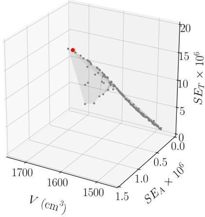
**Fig. 9:** Pareto front [grey scatter] where the shielding efficiencies axial,  $SE_A$ , and transverse,  $SE_T$ , to the shield's axis are maximized and total volume of shielding material,  $V$ , is minimized. Pareto-optimal solutions are filtered to maximize  $SE_A$  [chosen solution red].
