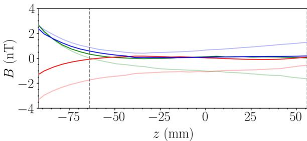
**Fig. 7:**  $B_x$ ,  $B_y$ , and  $B_z$  [green, red, and blue] along the  $z$ -axis of the inner shield cylinder with [solid] and without [light] static active background nulling between  $z = [-64, 56]$  mm [grey dashed lines].
