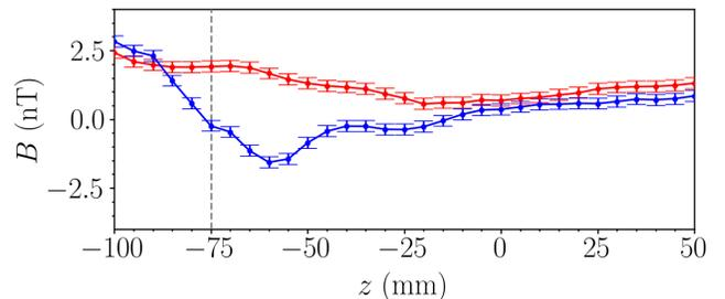
**Fig. 3:** Residual norm( $B_x, B_y$ ) and  $B_z$  measured along the  $z$ -axis of the inner shield cylinder using a fluxgate magnetometer [red and blue] inside a MSR. Dashed grey line shows the edge of the target field region.
