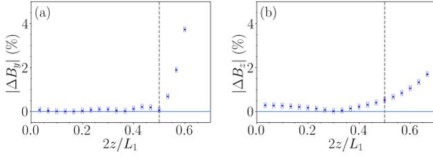
**Fig. 6:** Deviation between the measured and target fields for the uniform (a)  $B_y$  and (b)  $B_z$  flex-PCBs plotted versus position along the  $z$ -axis of the inner shield cylinder. Labelled as Fig. 5.
