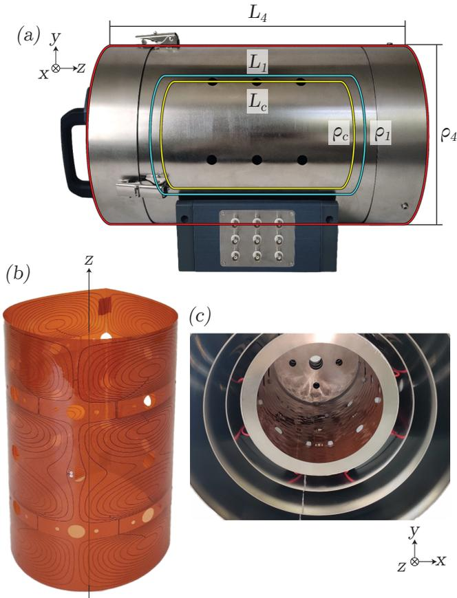
**Fig. 1:** The benchtop shield consists of four nested mumetal cylinders of outer radius  $\rho_4 = 150$  mm and length  $L_4 = 480$  mm [red] and inner radius  $\rho_1 = 100$  mm and length  $L_1 = 300$  mm [blue], which enclose a co-axial and co-centered set of rolled flex-PCBs of exterior radius  $\rho_c = 95$  mm and length  $L_c = 270$  mm [yellow]. (a) Side view of the shield and end caps, (b) a rolled PCB, and (c) multiple PCBs housed inside the shield with the end cap removed.
