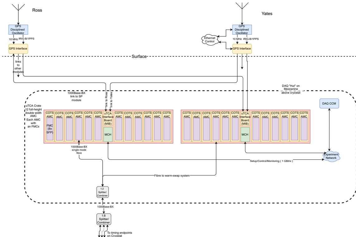
Figure 5. Schematic view of the DUNE timing system.
