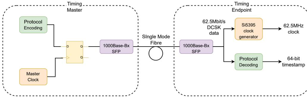
**Figure 3.** Block diagram of jitter performance test setup.
