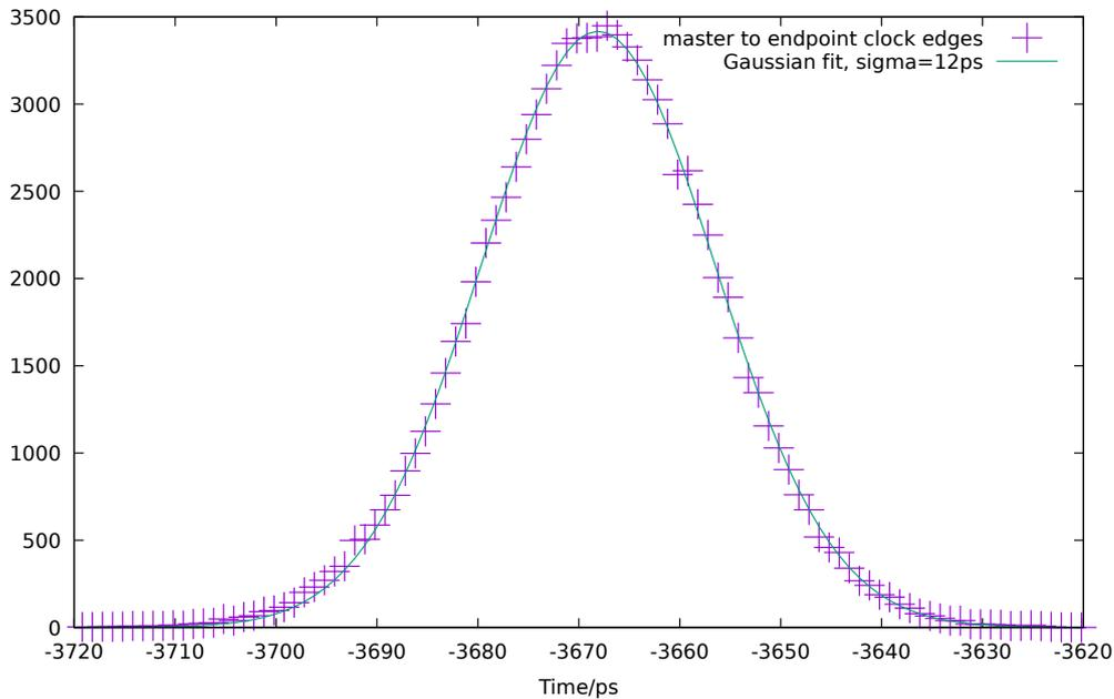
**Figure 4.** Distribution of time difference between clock edges at timing master and endpoint.
