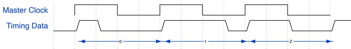
**Figure 1.** Illustration of Duty Cycle Shift Keying (DCSK) showing the representation of '0', '1' and 'Z' values.
