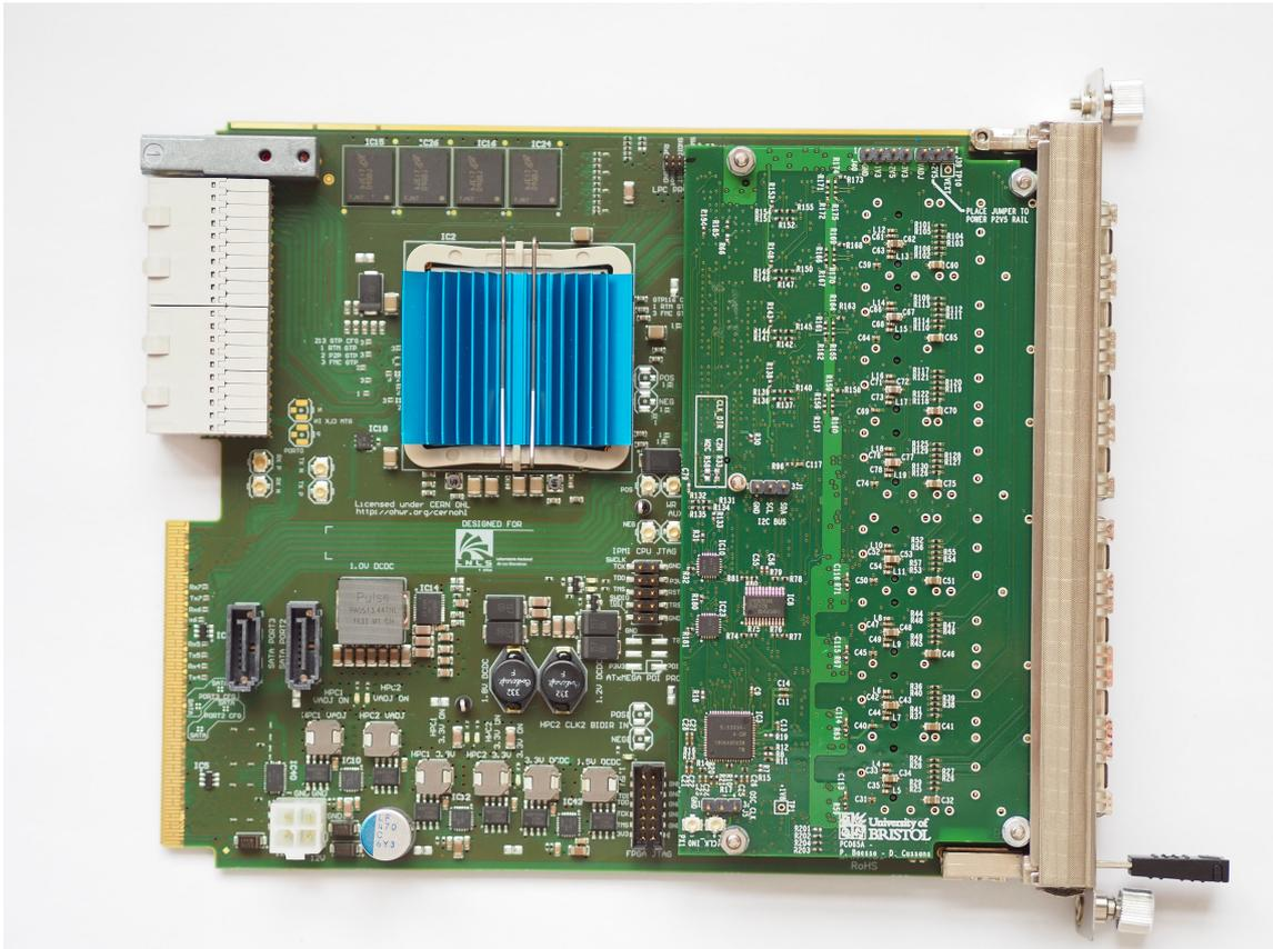
**Figure 6.** Photograph of a DUNE timing system Fibre Interface Board mounted on a commercial FPGA based AMC.
