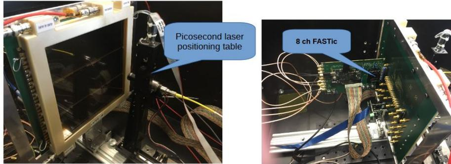
**Figure 3.** Image of the LAPPD detector in the setup, image of the anode plane with FASTic and PETsys attached electronics.
