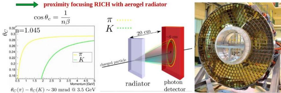
**Figure 1.** Kaon and Pion Cherenkov angle emission as a function of particle momentum. RICH detector configuration using Aerogel as radiator, and image of the Belle II ARICH detector installed at Belle II spectrometer.
