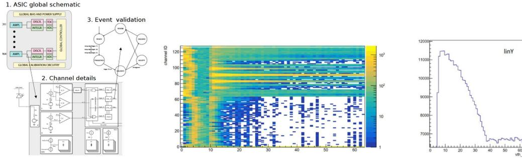
**Figure 4.** Block schematic of the ASIC, calibrated threshold scan with channel 91 illuminated (Y-channel, X-Threshold, Z-Magnitude), and threshold scan profile of channel 91, counts as a function of threshold.
