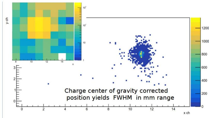
**Figure 6.** Left top is binary histogrammed output illuminating channel 91, and right is the recalculated position using the center of gravity estimation. One unit is equivalent to 6 mm.
