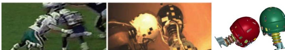
Figure 4: **Impact reconstruction:** From game video analysis (on the left) to laboratory re-enactments (centre) to virtual simulation (right) of a real concussive impact in American Football [14]
