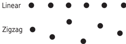
FIG. 2. Structure of 6 ions in the linear Paul trap. When the anisotropy is 6.8, the transverse confinement is much stronger than the axial confinement, the ion string stays linear structure. Damping the transverse confinement with constant axial confinement, which reduces the anisotropy to 3.4, the ion undergoes a structural phase transition from the linear to zigzag.
