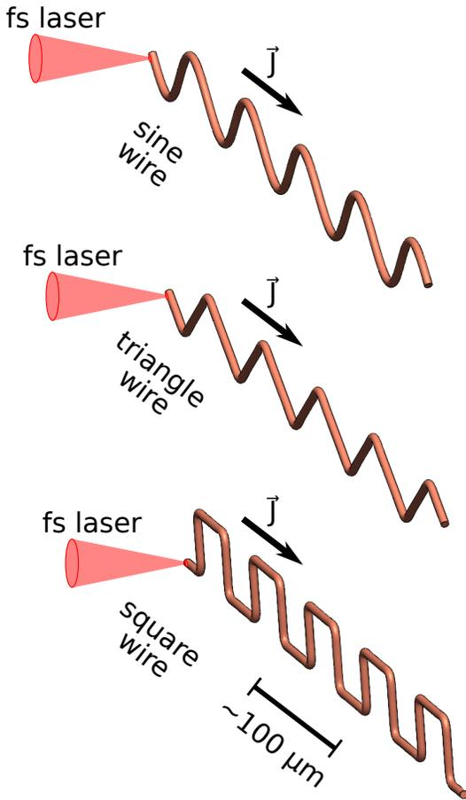
FIG. 1. Sketch of the proposed targets: 'sine' wire (top), 'triangle' wire (middle) and 'square' wire (bottom). The targets are irradiated on the open end by an intense femtosecond laser pulse. The general propagation direction of the laser-induced discharge pulse is shown with black arrows - it propagates from the irradiated end of the wire to the opposite one along the wire surface.
