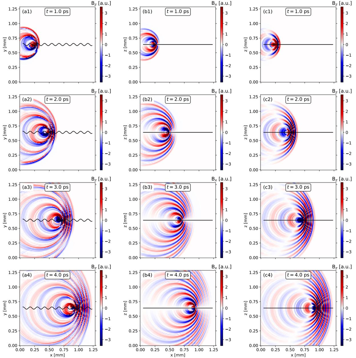
FIG. 3. Electromagnetic fields emitted by the 'sine' target with geometry defined by Eq. 1: (a1-a4)  $B_z$  component in the plane of the target, i.e. at  $z = 0.64$  mm, at time moments 1.0, 2.0, 3.0 and 4.0 ps, respectively; (b1-b4)  $B_x$  component in  $y = 0.64$  mm plane at the same time moments; (c1-c4)  $B_z$  component in  $y = 0.64$  mm plane at the same time moments. The projections of the target on the considered planes are shown with solid black lines.
