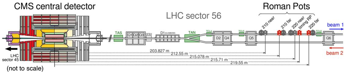
Figure 2: A schematic layout of one arm of CT-PPS along the LHC beam line. The RPs shown in red are those used by CT-PPS; those in grey are part of the TOTEM experiment. From [2].
