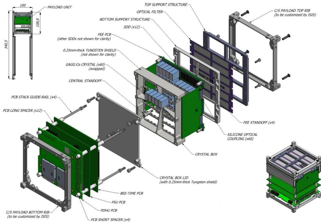
Figure 1: Exploded view of the HERMES Payload (P/L).
