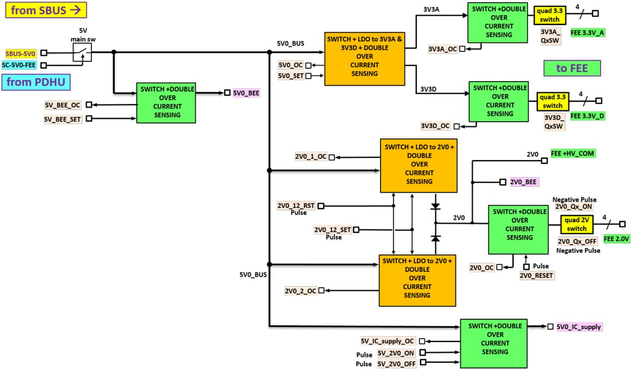
Figure 7: Block diagram representation of HERMES-PSU 5V0 section.
