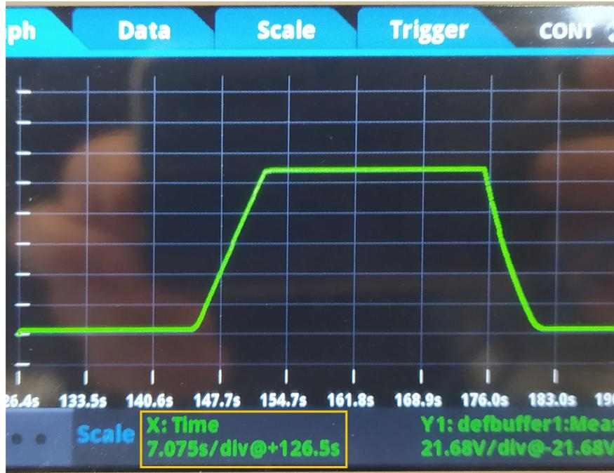
Figure 12: Ramp-HV curve
