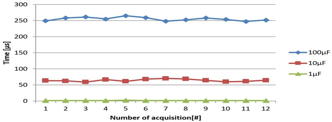
Figure 14: Variation in OC detection time when varying load capacity
