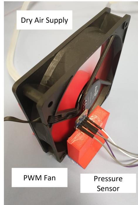
Fig. 8. Test setup was built using 3D printed parts which have a cavity for dry air supply and a surface to fix the pressure sensor.
